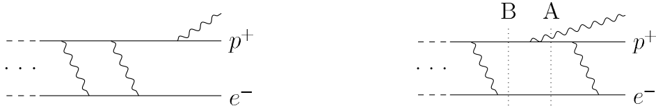
Figure 6. Bremsstrahlung diagrams. On the dotted line A, there are two fermions and one photon. On the other hand, on the dotted line B, there are only two fermions.
