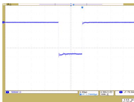
Fig.6 The gun current signal from oscilloscope
