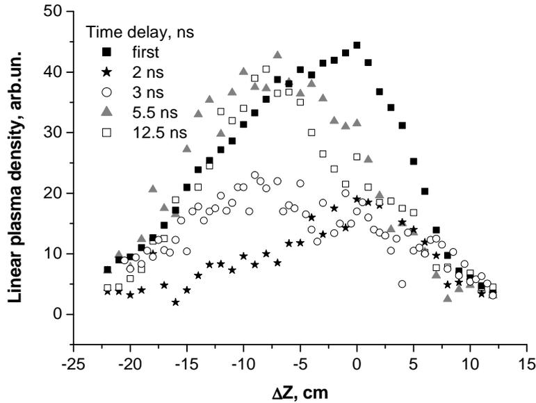
Fig.2. Linear plasma density v.s. distance  $\Delta Z = F - Z$  (Z-coordinate of the plasma channel along the optical axis, F - focal length) for the first UV laser pulse and the second one for various time delays between them. Laser radiation goes from the left side.
