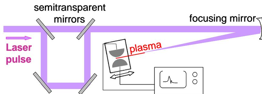
Fig. 1. Scheme of registration of the electron plasma formed by a double femtosecond pulse.
