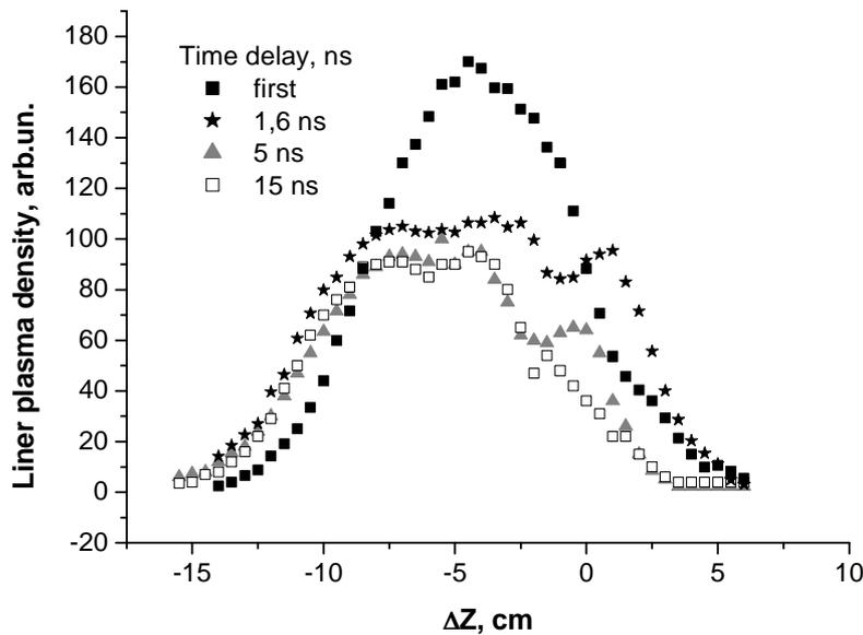
Fig. 3. Linear plasma density v.s. distance  $\Delta Z = F - Z$  (Z-coordinate of the plasma channel along the optical axis, F - focal length) for the first IR laser pulse and the second one for various time delays between them. Laser radiation goes from the left side.
