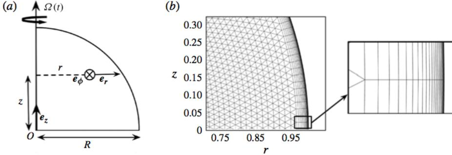
FIGURE 1. (a) Schematic of the upper quarter of the sphere with the cylindrical polar vectors ( $\mathbf{e}_r, \mathbf{e}_\phi, \mathbf{e}_z$ ). (b) Mesh grid used in the numerical model showing two zones: a bulk zone with triangular elements and a boundary-layer domain with quadrangular elements. The inset is a zoom of the mesh grid near the outer boundary.
