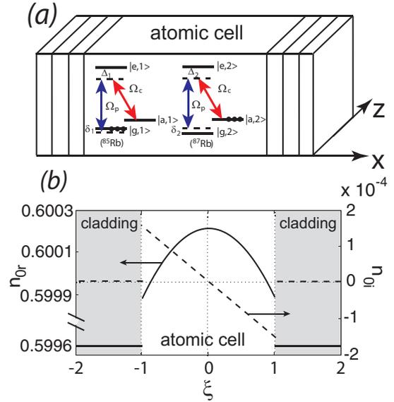
Fig. 1. (Color online) (a) Geometry of the photonic crystal, the energy-level diagram, and Raman resonance scheme of a binary mixture. The initially populated levels are indicated by the black dots. (b) Distribution of real  $n_{or}$  (solid line) and imaginary  $n_{oi}$  (dashed line) parts of the linear refractive index induced by the fields (4).
