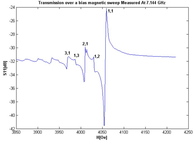
Fig. 14. The Fano-interference effect in a microwave microstrip structure obtained by varying a bias field at a constant frequency  $f = 7.144\text{GHz}$ . In the mode designation, the first number characterizes a number of radial variations for the MDM spectral solution. The second number is a number of azimuthal variations for the MDM spectral solution [16].
