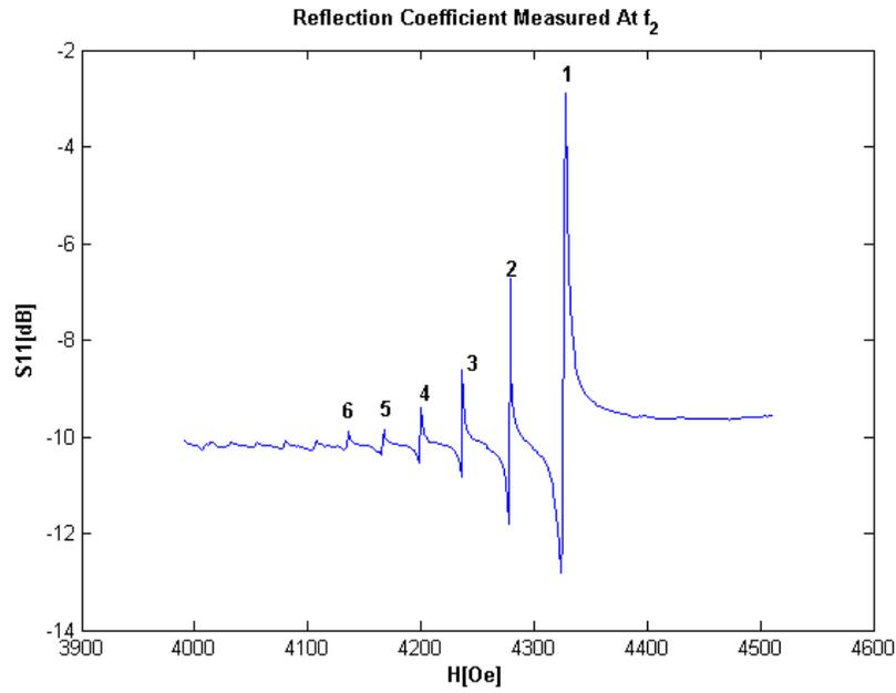
Fig. 10. The Fano-interference effect in a  $TE_{102}$ - mode waveguide cavity with an embedded normally magnetized MDM ferrite disk at frequency  $f_2 = 7.49GHz$ .
