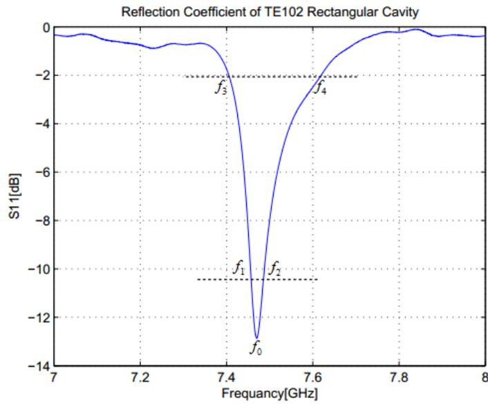
Fig. 8. The cavity resonant characteristics. The quantities of the frequencies:  $f_0 = 7.4731\text{GHz}$ ,  $f_1 = 7.4575\text{GHz}$ ,  $f_2 = 7.49\text{GHz}$ ,  $f_3 = 7.4081\text{GHz}$ ,  $f_4 = 7.6188\text{GHz}$ .
