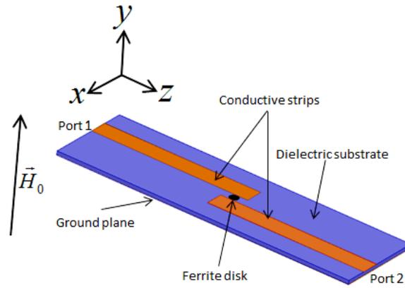
Fig. 13. A microstrip structure with an embedded MDM ferrite disk.
