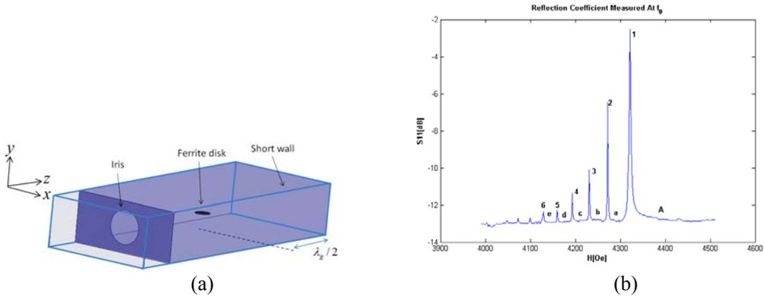
Fig. 2. MDM resonances in a microwave cavity. (a) A  $TE_{102}$ -mode rectangular waveguide cavity with a normally magnetized ferrite-disk sample; (b) An experimental multiresonance spectrum of modulus of the reflection coefficient obtained by varying a bias magnetic field and at a resonant frequency of  $f_0 = 7.4731\text{GHz}$ . The resonance modes are designated in succession by numbers  $n = 1, 2, 3, \dots$ . The states beyond resonances we designate with small letters  $a, b, c, \dots$
