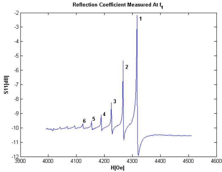
Fig. 9. The Fano-interference effect in a  $\text{TE}_{102}$ - mode waveguide cavity with an embedded normally magnetized MDM ferrite disk at frequency  $f_1 = 7.4575\text{GHz}$ . The MDM resonances are designated by numbers  $n = 1, 2, 3, \dots$
