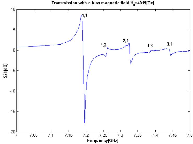
Fig. 15. The Fano-interference effect in a microwave microstrip structure obtained by varying signal frequency at a constant bias field  $H_0 = 4015\text{Oe}$ . In the mode designation, the first number characterizes a number of radial variations for the MDM spectral solution. The second number is a number of azimuthal variations for the MDM spectral solution [16].
