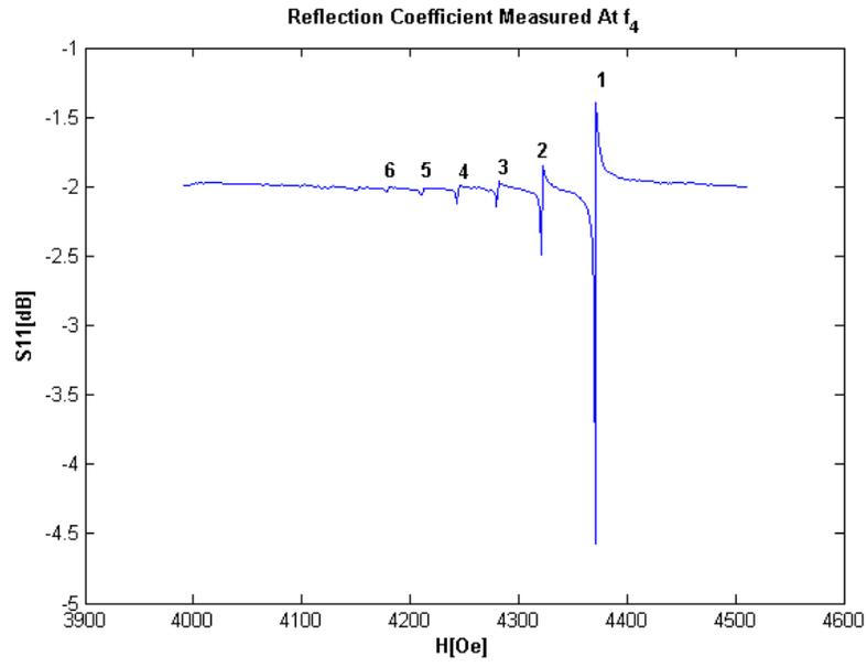
Fig. 12. The Fano-interference effect in a  $TE_{102}$ - mode waveguide cavity with an embedded normally magnetized MDM ferrite disk at frequency  $f_4 = 7.6188GHz$ .
