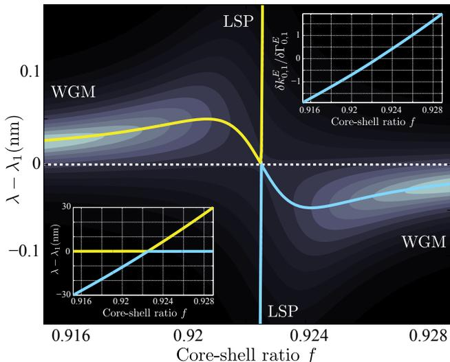
FIG. 1: (Color online) Normalised extinction spectrum vs. ratio of core-shell radii for a coupled WGMR-NP system illuminated to excite the (40, 1) WGM in a bare WGMR. Solid lines show resonance branches defined by Eq. (9). Left inset: larger scale view of resonance branches. Right inset: ratio of resonance shift,  $\delta k_{0,1}^E$ , to line broadening,  $\delta \Gamma_{0,1}^E$ , quantifying reactive vs resistive coupling.
