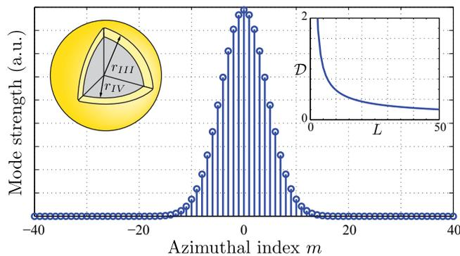
FIG. 2: (Color online) Mode strengths of degenerate azimuthal modes in a fundamental  $L = 40$  WGM. Left inset: geometry of a core-shell NP. Right inset: variation of the ratio  $D = \sum_{|m| \le 1} |D_m|^2 / \sum_{2 \le |m| \le L} |D_m|^2$  with polar index  $L$ .
