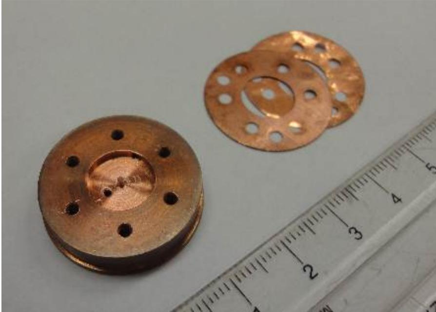
Fig. 5. Photograph of the copper cavity and gaskets for the re-entrant cavity under investigation.
