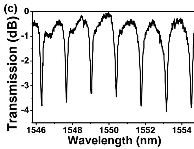
**Figure 5.** Direct Monolithic Imprint Fabrication on Nonplanar Substrates. (a) A photo showing imprinted ChG resonator devices on a flexible PET substrate; (b) top-view microscope image of ChG ring resonators imprinted on a flexible polyimide film; (c) transmission spectrum of an imprinted  $\text{As}_{20}\text{Se}_{80}$  micro-ring resonator on a flexible substrate: an average  $Q = 10,000$  was measured.
