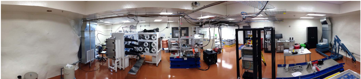
FIG. 11: A view of the detector laboratory at the Davis Campus at SURF. In this view, the glove box is to the left, and the prototype module is center. In the rear, a soft-wall cleanroom is shown that serves the purpose of an area of increased cleanliness.
