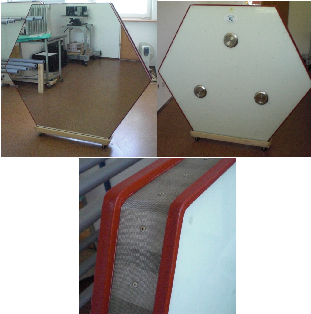
Figure 2: The front of an open structure mirror with reflective layer (top left) and the rear side with mounting pads (top right). Visible are the protective silicon rubber and stainless steel mesh (bottom panel).
