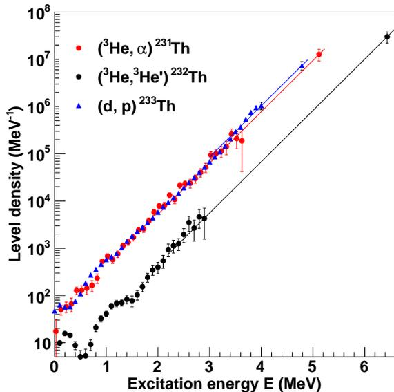
FIG. 5: (Color online) Level densities for  $^{231-233}\text{Th}$  for the reactions with best statistics. The constant temperature extrapolations (solid lines) were calculated with  $T_{\text{CT}} = 0.40$  MeV.
