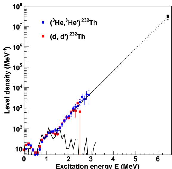
FIG. 4: (Color online) Normalization of the nuclear level density of  $^{232}\text{Th}$  for the  $(^3\text{He},^3\text{He}')$  and  $(d,d')$  reactions. See text of Fig. 3.
