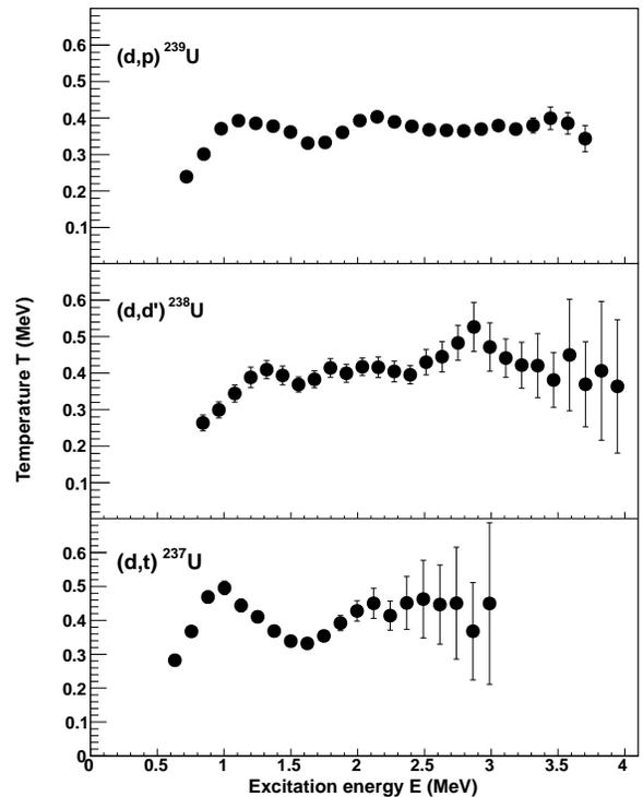
FIG. 8: Microcanonical temperatures for  $^{237-239}\text{U}$  as function of excitation energy from this work.
