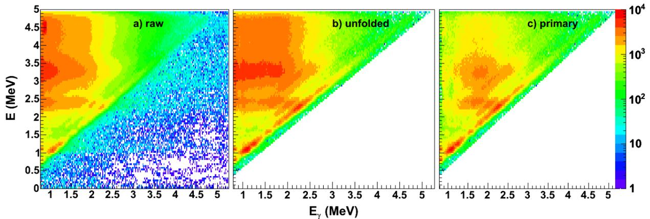
FIG. 1: (Color online) Initial excitation energy  $E$  versus  $\gamma$ -ray energy  $E_\gamma$  from particle- $\gamma$  coincidences recorded with the  $^{232}\text{Th}(d,p\gamma)^{233}\text{Th}$  reaction. The raw  $\gamma$ -ray spectra (a) are first unfolded (b) by the NaI response function. In the last step (c), the primary or first-generation  $\gamma$ -ray spectra are extracted as function of excitation energy  $E$ .
