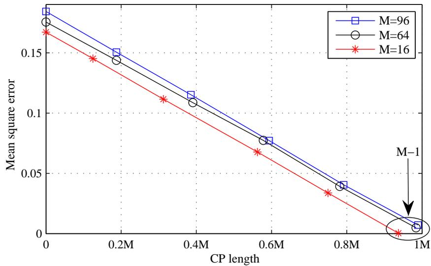
Fig. 10. The mean square errors for insufficient CP lengths.
