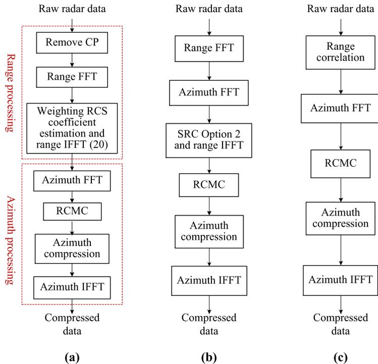
Fig. 5. Block diagram of SAR imaging processing: (a) CP based OFDM SAR; (b) LFM SAR; (c) Random noise SAR and conventional OFDM SAR.
