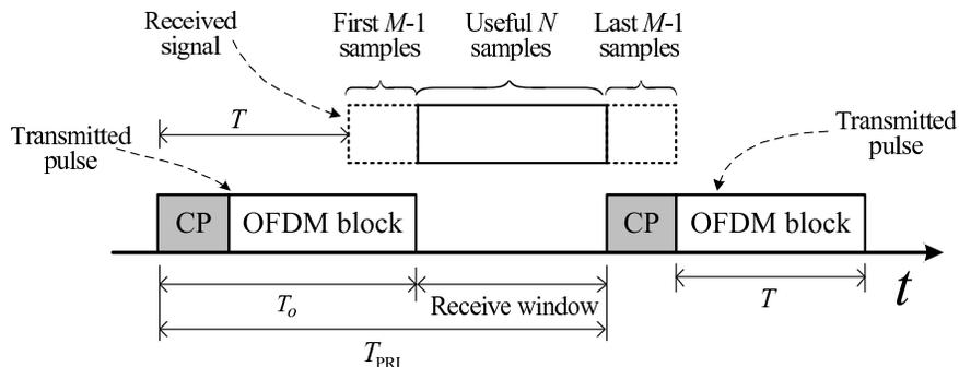
Fig. 4. Transmitted and received timing of OFDM SAR system for  $M = N$ .
