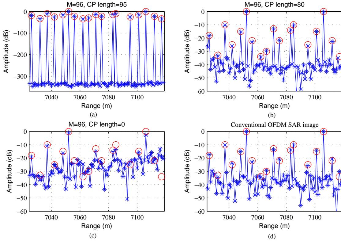
Fig. 9. A range line imaging with different CP lengths. Red circles denote the real target amplitudes, blue asterisks denote imaging results.
