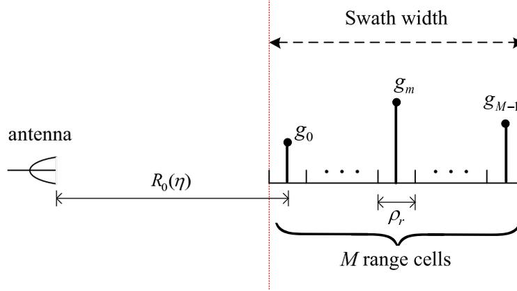
Fig. 2. Illustration diagram of one range line.
