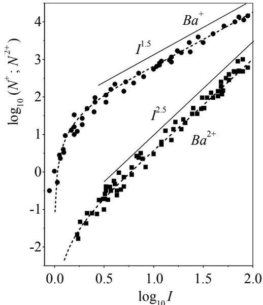
FIG. 5: Dependence of the  $Ba^+$  and  $Ba^{2+}$  yields on the intensity  $I$  of color-centre laser radiation at the frequency  $\omega = 8865\text{cm}^{-1}$ . Points denote experimental measurements. Dashed lines represent experimental data fits by  $V_0(I)$  [equation (3)] for  $Ba^+$  and by  $IV_0(I)$  for  $Ba^{2+}$ , respectively. For comparison, the power laws  $N^+ \sim I^{1.5}$  and  $N^{2+} \sim I^{2.5}$  are displayed by solid lines.
