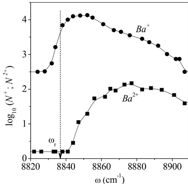
FIG. 1: Dependences of the singly and doubly charged ion yields on the laser radiation frequency for Ba atom ionization with color-centre laser radiation. The dashed vertical line denotes the frequency of the four-photon excitation of the unperturbed state  $6p^2\ ^1D_2$  ( $\omega_r = 8836\text{cm}^{-1}$ ).
