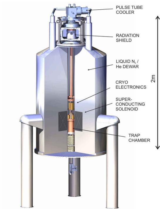
FIG. 6. (Color online) Schematic drawing of the setup. The superconducting magnet has been cut to allow a view of the trap and related components inside the room-temperature bore.
