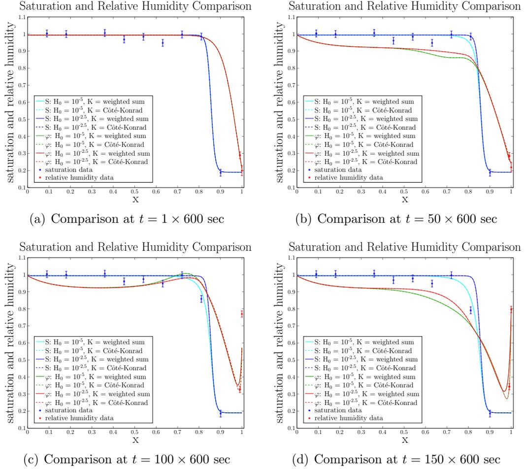
Figure 7.19: Comparison of relative humidity and saturation for the fully coupled saturation-diffusion-temperature model as compared to data from [75]. Boundary conditions are taken from a sinusoidal approximation of boundary data. Thermal conductivities are taken as either weighted sum (5.78) or Côté-Konrad (5.80).
