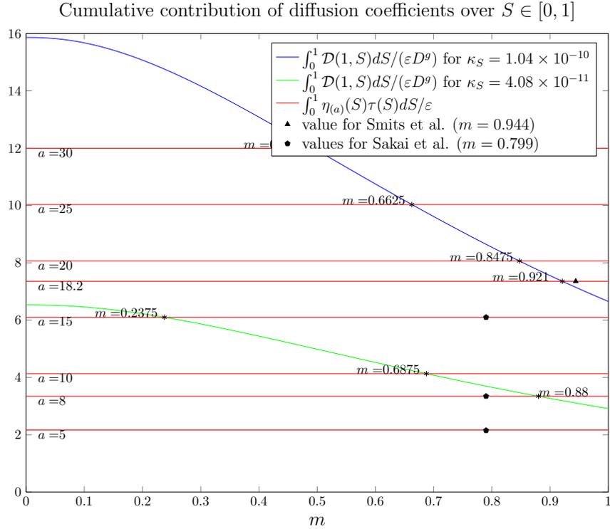
Figure 7.10: The blue and green curves show the left-hand side of equation (7.8) for different saturated permeabilities, and the red lines show level curves for right-hand side for various values of  $a$ . The blue and green curves can be used to predict the value of  $a$  before experimentation.
