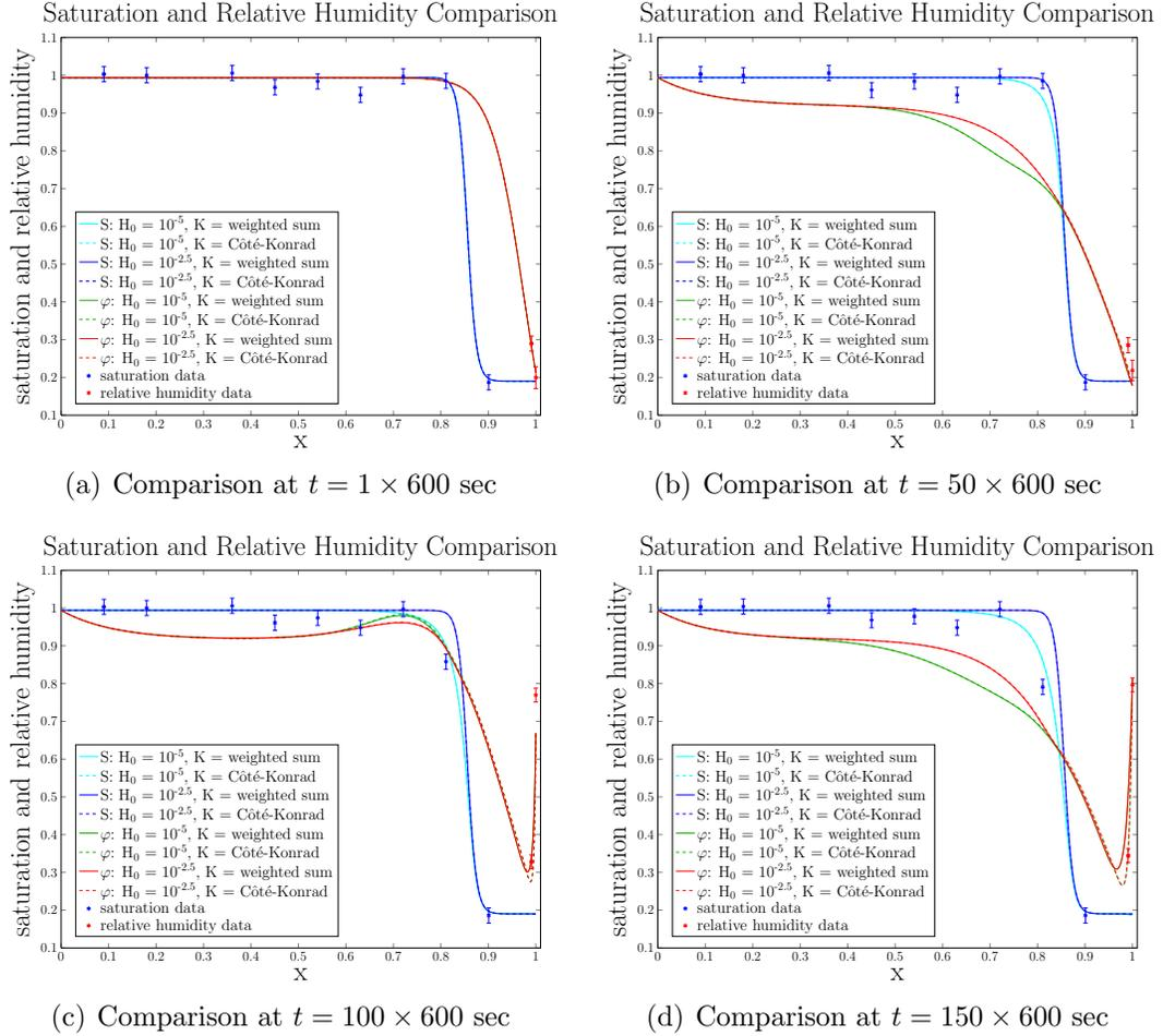
Figure 7.20: Comparison of relative humidity and saturation for the fully coupled saturation-diffusion-temperature model as compared to data from [75]. Boundary conditions are taken from a smoothed square wave approximation of boundary data. Thermal conductivities are taken as either weighted sum (5.78) or Côté-Konrad (5.80).
