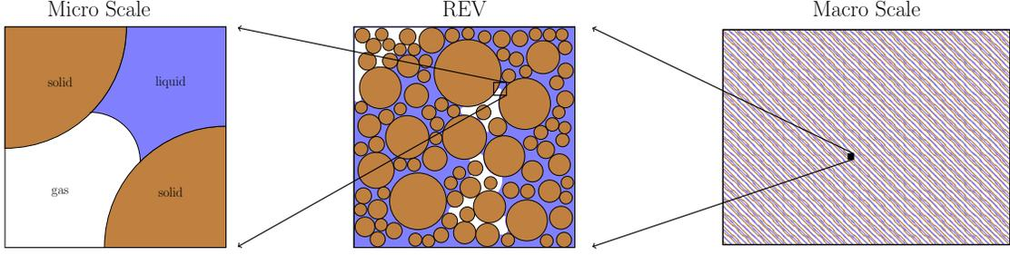
Figure 3.2: Cartoon of the microscale, REV, and macroscale in a granular soil. The right-hand plot depicts the mixture of all phases.
