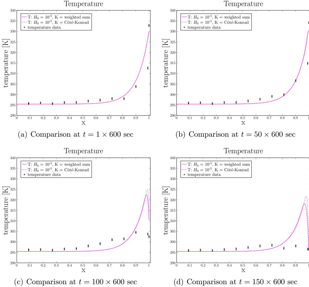
Figure 7.22: Comparison of temperature solutions for the fully coupled saturation-diffusion-temperature model as compared to data from [75]. Boundary conditions are taken from a sinusoidal approximation of boundary data.
