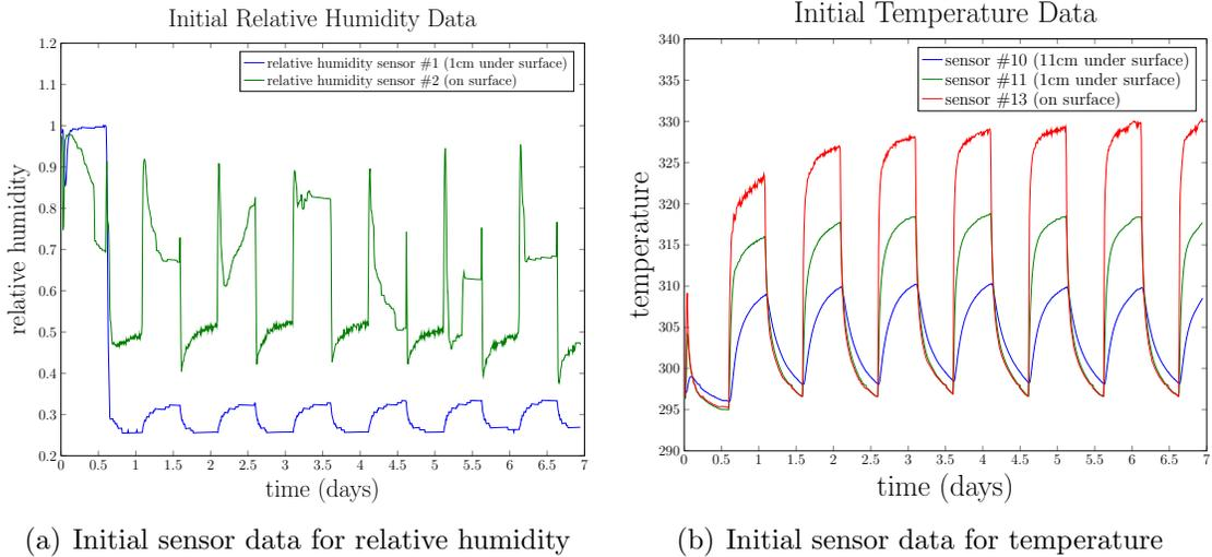
Figure 7.14: Relative humidity and temperature data showing measurement variations in the first few days of the experiment. (Image recreated with permission from [75])
