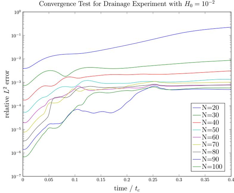
Figure 7.4: Convergence test for drainage experiment depicted in Figure 7.3.  $N$  is the number of spatial grid points. In Figure 7.3,  $t_1 = 0.025t_c$ ,  $t_2 = 0.050t_c$ ,  $t_3 = 0.075t_c$ , and  $t_4 = 0.10t_c$
