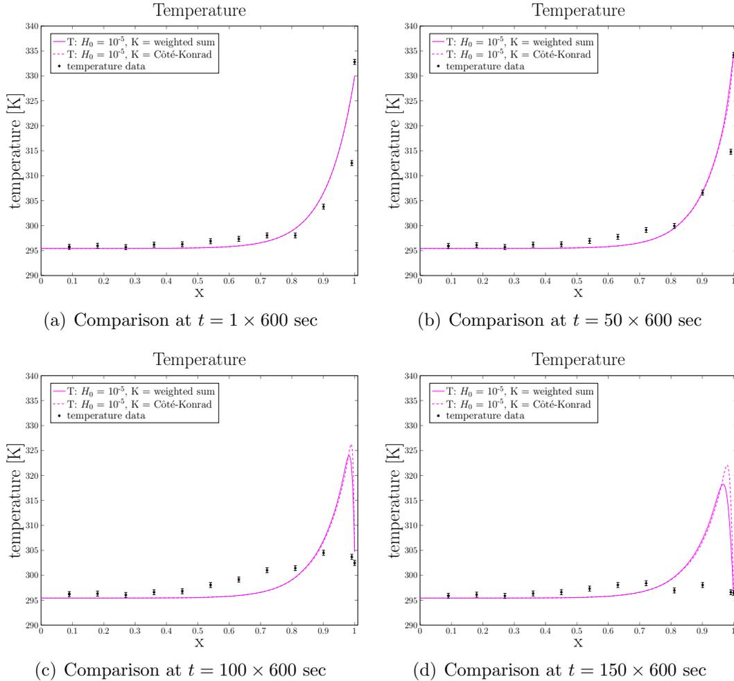
Figure 7.23: Comparison of temperature solutions for the fully coupled saturation-diffusion-temperature model as compared to data from [75]. Boundary conditions are taken from a smoothed square wave approximation of boundary data.
