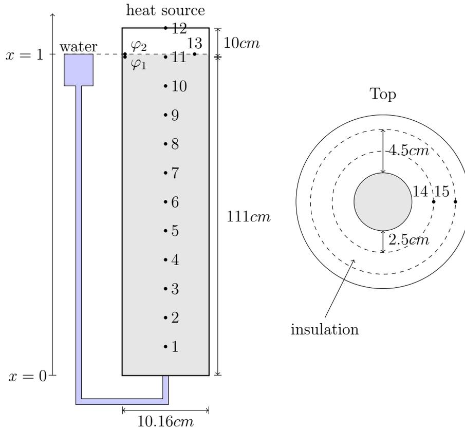
Figure 7.12: Schematic of the Smits et al. experimental apparatus. Saturation and temperature sensors numbered 1 - 11, temperature sensors 12 - 15, and relative humidity sensors 1 and 2 [75]. The geometric  $x$  coordinate is shown on the left. (Image recreated with permission from [75])
