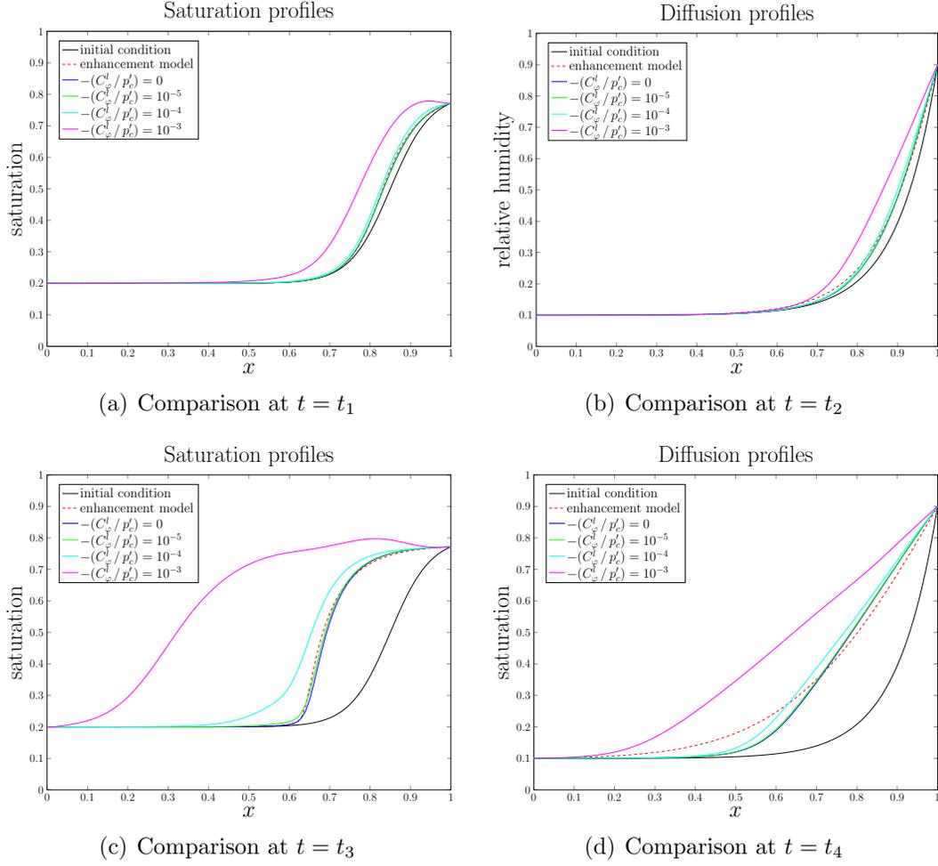
Figure 7.11: Comparison of coupled saturation-diffusion models for various weights of  $C_\varphi^l$  with parameters:  $\kappa_s = 1.04 \times 10^{-10}$ ,  $\varepsilon = 0.334$ ,  $H_0 = 10^{-3}$ ,  $\alpha = 4$ , and  $m = 0.667$ .
