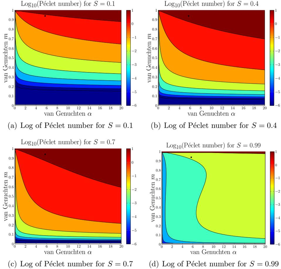
Figure 7.2: Log of Péclet numbers for various values of saturation. The point at  $(\alpha = 5.7, m = 0.94)$  indicates the values used in Smits et al. [75]. Warmer colors are associated with higher Péclet number and therefore associated with an advective solution.
