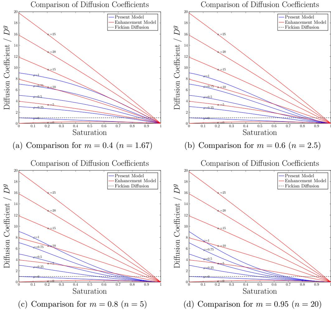
Figure 7.9: Comparison of diffusion coefficients for various van Genuchten parameters all taken with  $\kappa_s = 4.0822 \times 10^{-11}$  and  $\varepsilon = 0.385$  to match the experiment in [67].
