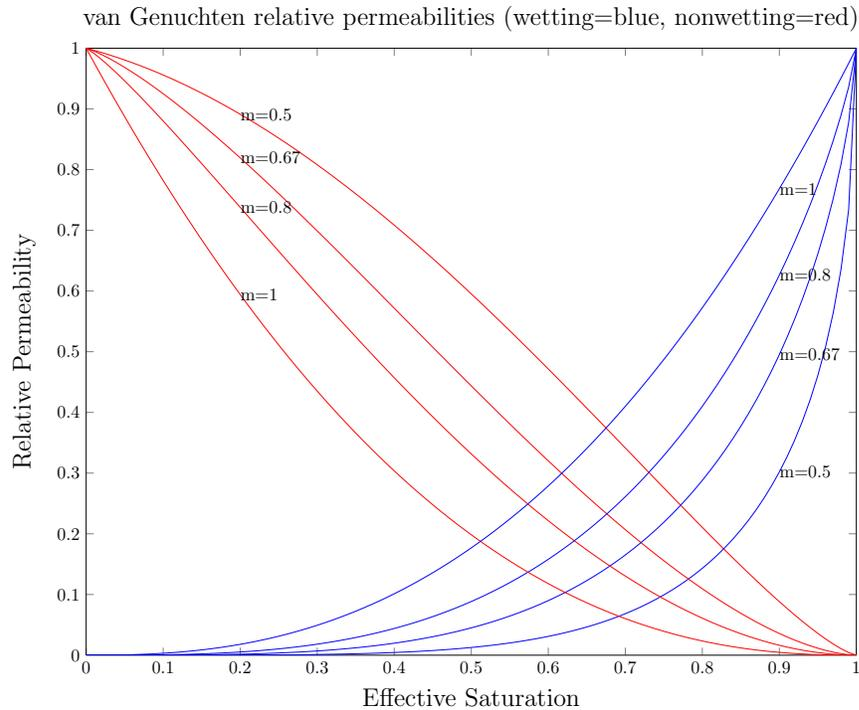
Figure 5.2: van Genuchten relative permeability curves. The red curve shows the non-wetting phase,  $\kappa_{r_{nw}}(S_e)$ , and the blue curves show the wetting phase,  $\kappa_{r_w}(S_e)$ , each for  $m = 0.5, 0.67, 0.8$ , and  $1$ .
