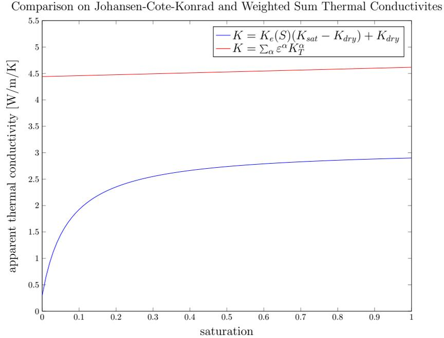
Figure 5.6: Johansen thermal conductivity model with Côté-Konrad  $K_e - S$  relationship (with  $\kappa = 15$ ) plotted in blue, and the weighted sum of the thermal conductivities of the individual phases plotted in red.
