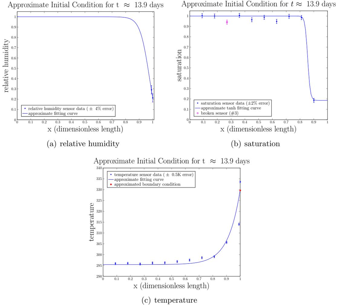
Figure 7.17: Approximate initial conditions at the 2000<sup>th</sup> data point ( $t \approx 13.9$  days). Error bars indicate approximate sensor accuracy.
