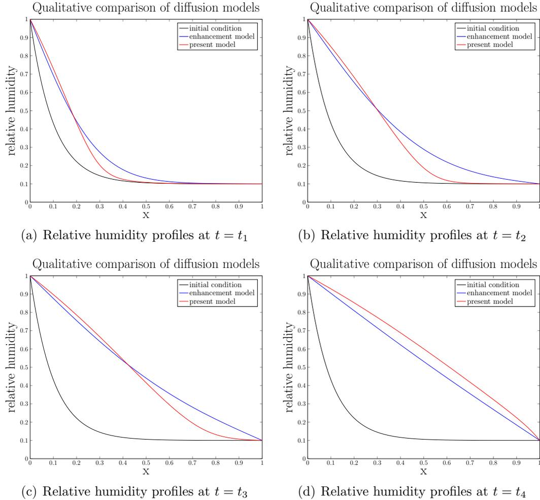
Figure 7.7: Sample diffusion experiment comparing the enhancement model to the present model. Here,  $a = 25$ ,  $m = 0.9$  ( $n = 10$ ), and  $\kappa = 10^{-10}$  with Dirichlet boundary conditions and an exponential initial profile.
