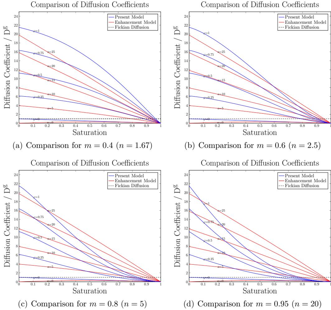
Figure 7.8: Comparison of diffusion coefficients for various van Genuchten parameters all taken with  $\kappa_s = 1.04 \times 10^{-10}$  and  $\varepsilon = 0.334$  to match the experiment in [75].
