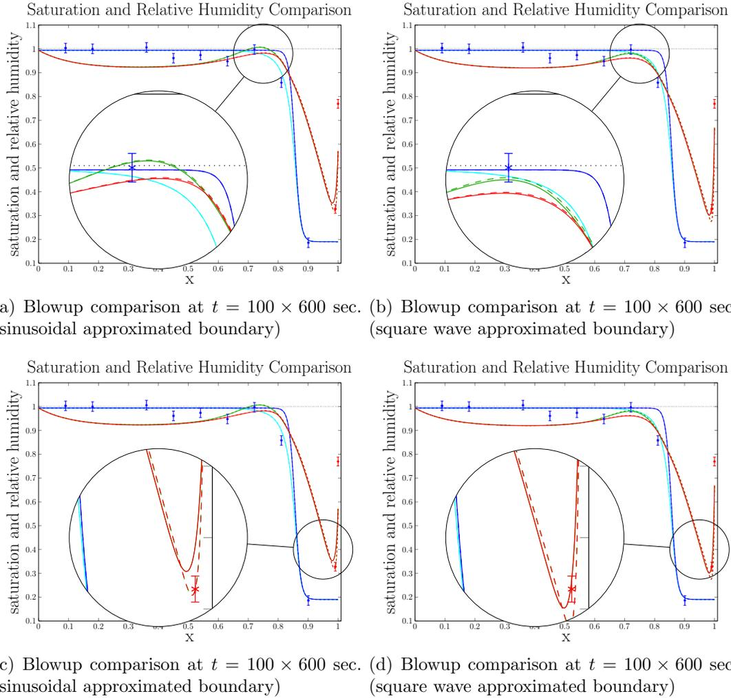
Figure 7.21: Blowup comparison of relative humidity and saturation for the fully coupled saturation-diffusion-temperature model as compared to data from [75]. The inset plots give a closer look at the behavior exhibited by these particular solutions.
