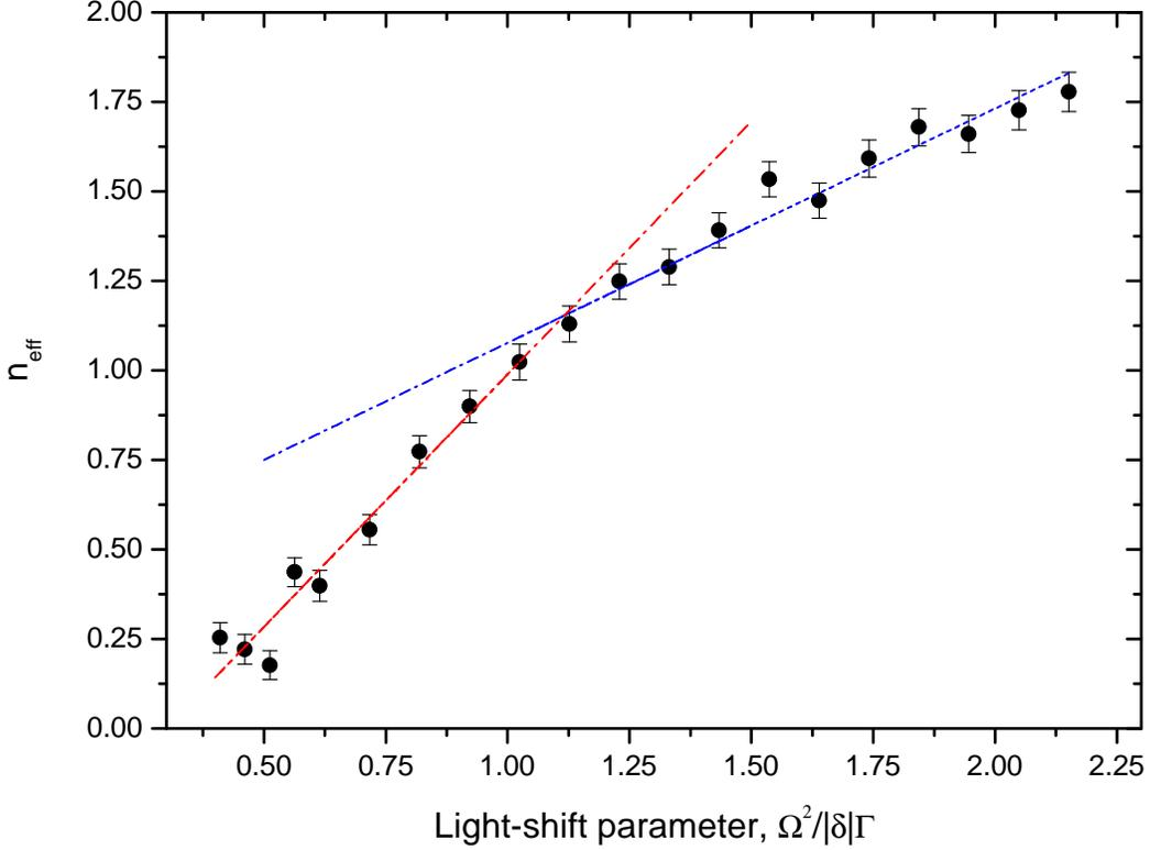
Figure 7: Estimation of effective atom-number,  $n_{eff}$ , with increasing dimensionless light-shift parameter  $\Omega^2/|\delta|\Gamma$  (black circles) with two linear fits to indicate the change in slope around a light-shift parameter 1.2.
