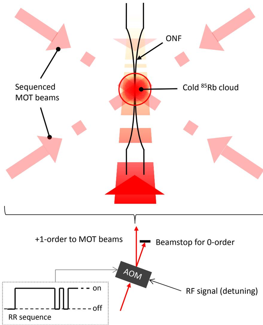
Figure 2: Illustration of the experimental setup. The 1<sup>st</sup>-order beam from an AOM is expanded and split into three equal-intensity cooling beams for the MOT. The  $^{85}\text{Rb}$  cloud is positioned centrally around the ONF. The cooling beams are switched on and off according to the sequence shown here with an AOM. Beam detuning is controlled via the tunable RF input on the AOM.
