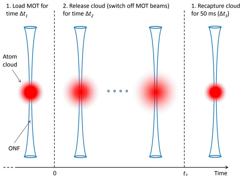
Figure 1: Illustration of the release and recapture sequence as a function of time. The cloud is positioned centrally around the ONF. The cloud is loaded for a time  $\Delta t_1$  and then released from the trap for a time  $\Delta t_2$ .  $\Delta t_2$  is varied from sequence to sequence to build up a profile of the velocity of the atoms in the MOT. The recapture time,  $\Delta t_3$ , is set to 50 ms. The cloud is then released once more for 50 ms, before repeating the entire sequence.
