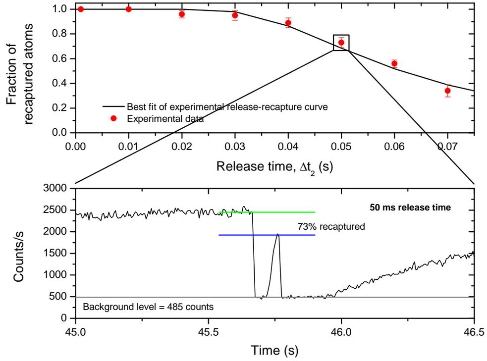
Figure 3: Fraction of recaptured atoms estimated from the fluorescence data obtained from an optical nanofibre placed near the cold cloud of atoms. For a release time,  $\Delta t_2$ , of 50 ms, 73% of the expanded cloud was recaptured with  $\delta=-2.6\Gamma$  and cooling laser intensity of  $2.9I_s$  ( $4.6 \text{ mW/cm}^2$ ) per beam.
