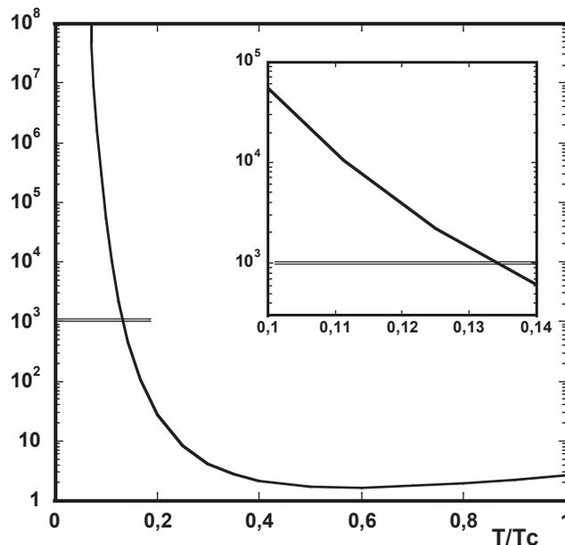
FIG. 1: The ratio of the Majorana heat capacity to that of the quasiparticles  $F$  from equation (0.3)(solid line) and the experimental parameter  $\lambda/\xi$  for a suggested experimental cell (double line)
