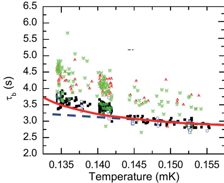
FIG. 2: The time constant of the Dark Matter detector measured after heat pulses  $\circ$ , neutrons (squares) and muons. For details see [7]. The dashed line shows the theoretical dependance for the bulk quasiparticle heat capacity and solid line that with the Majorana part taken into account.
