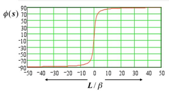
**Fig. 16:** Phase advance in a symmetric drift space as a function of the drift length
