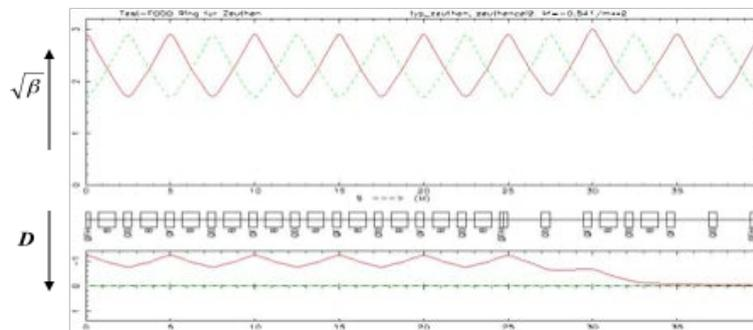
Fig. 21: Dispersion suppressor based on a missing-magnet scheme
