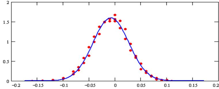
**Fig. 7:** Transverse beam profile of a HERA proton bunch at the interaction point. The measurement was performed by scanning the colliding beams against each other. The data points (dots) have been fitted by a Gaussian curve (line).
