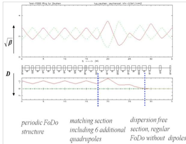
**Fig. 18:** Dispersion suppressor using individually powered quadrupole lenses
