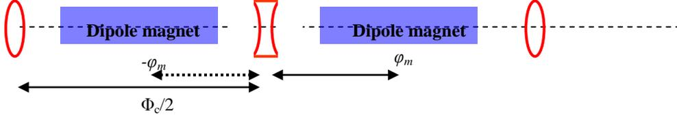
**Fig. 19:** Schematic view of a FODO: notation for the phase relations in the cell
