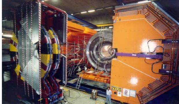
**Fig. 13:** Particle detector for the ZEUS collaboration at the HERA storage ring
