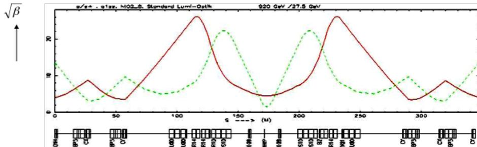
**Fig. 14:** Layout of a mini-beta insertion scheme
