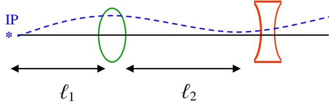
**Fig. 15:** Schematic layout of a mini-beta doublet
