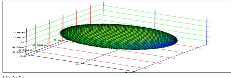
**Fig. 6:** Typical shape of a proton bunch in an arc of the HERA proton ring
