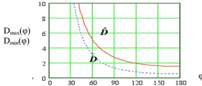
**Fig. 11:** Dispersion at the focusing and defocusing quadrupole lenses in a FODO as a function of the phase  $\varphi$
