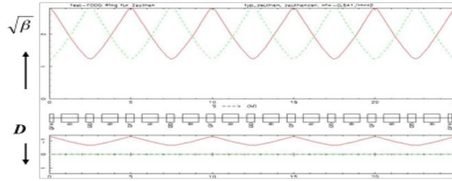
**Fig. 17:** Periodic FODO, including the horizontal dispersion function in the lower part of the plot
