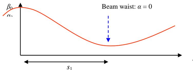
**Fig. 12:** Schematic drawing of a beam waist
