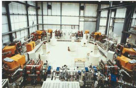
**Fig. 2:** The TSR heavy-ion storage ring at the Max-Planck-Institut in Heidelberg
