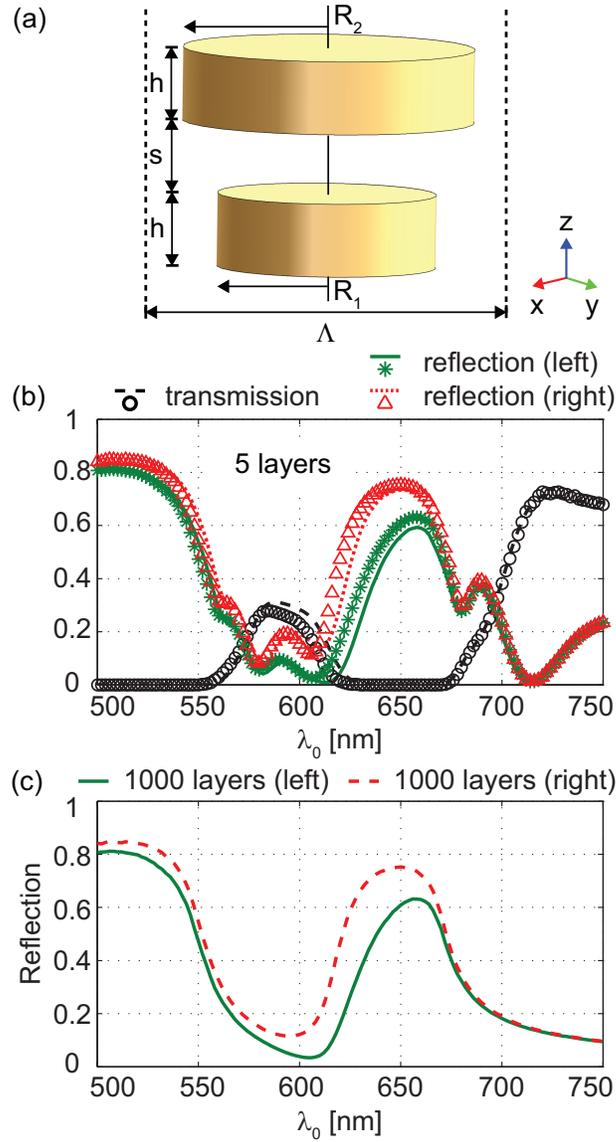
**Figure 5.** (a) Geometry of the disc nanodimer [ $2R_1 = 30$  nm,  $2R_2 = 40$  nm,  $h = s = 10$  nm,  $\Lambda = 50$  nm]. (b) is as in figure 3b. The numerically and analytically calculated reflections from the side of the larger discs are shown by the additional red dotted line and red triangles, respectively. (c) Reflection spectra for 1000 layers as obtained from (5) and (9).
