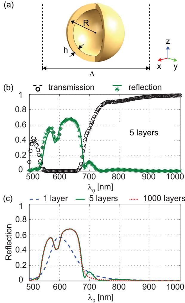
**Figure 3.** (a) Geometry of the nanoshell [ $2R = 70$  nm,  $h = 7$  nm,  $\Lambda = 130$  nm]. (b) Transmission and reflection spectra of a five-layer thick slab for TM-polarized incident light with the angle of incidence of  $45^\circ$ . The numerically calculated spectra (solid and dashed lines) are shown along with the analytical results (circles and stars) obtained from (5) and (9). (c) Reflection spectra for increasing number of layers as obtained from (5) and (9).
