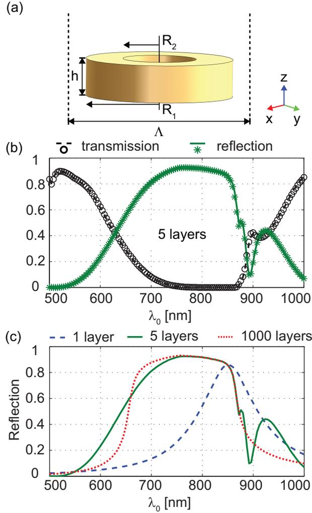
**Figure 4.** (a) Geometry of the nanoring [ $2R_1 = 40$  nm,  $2R_2 = 20$  nm,  $h = 10$  nm,  $\Lambda = 50$  nm]. (b) and (c) are as in figure 3.
