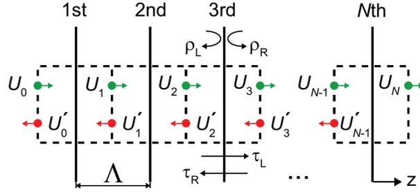
**Figure 2.** Light propagation through a metamaterial described by an array of infinitesimally thin sheets. Between each pair of such sheets there are two counter-propagating plane waves with transverse field components  $U_j$  and  $U'_j$ . The unit cells of the metamaterial are shown with dashed lines.
