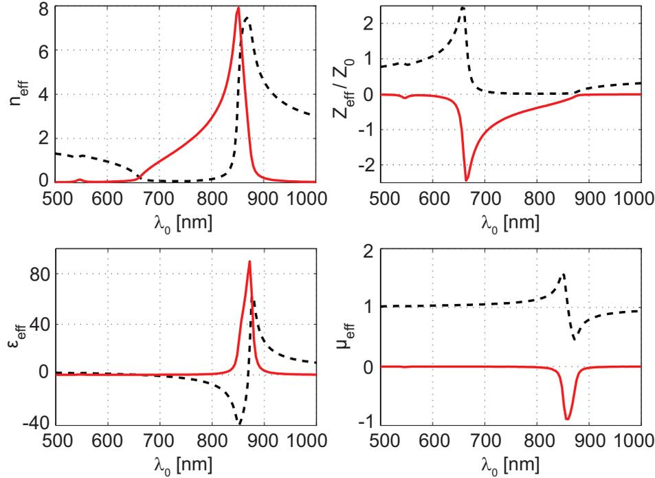
**Figure 6.** Real (black dashed lines) and imaginary parts (red solid lines) of the effective wave parameters for a material composed of the nanorings shown in figure 4. A TE-polarized wave propagating at  $\theta = 45^\circ$  in the host medium is considered.
