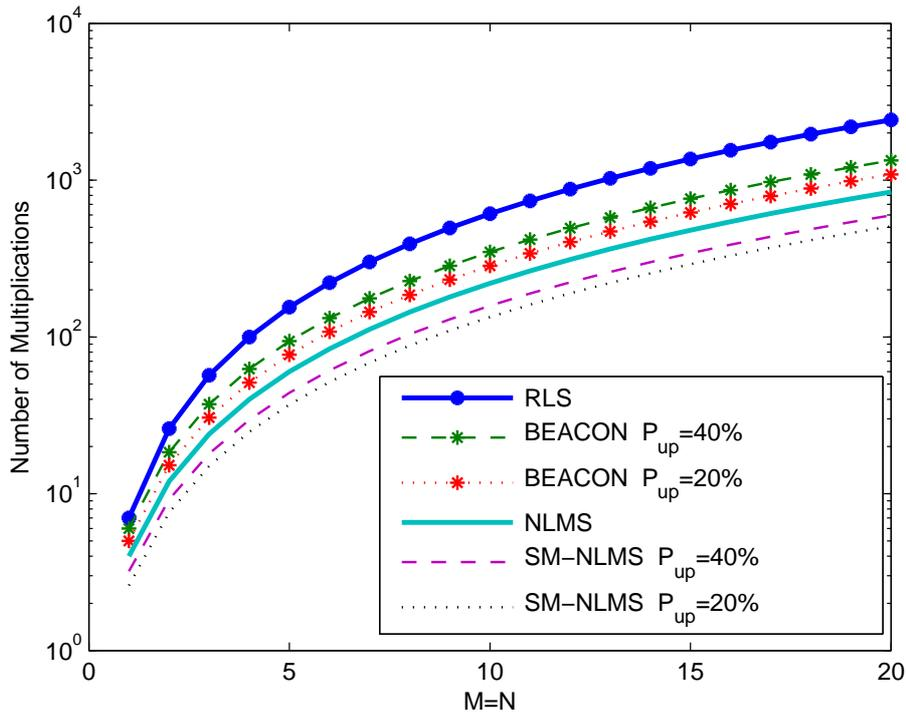
Fig. 4. The number of multiplications versus the size of the channel matrix.
