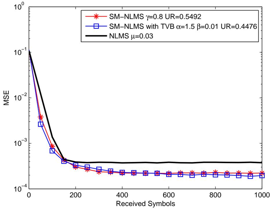
Fig. 7. MSE performance of the SM-NLMS channel estimation with a time-varying bound for quasi-static fading channel.  $n_p=1000$ ,  $n_t=100$  and  $n_d=900$ .
