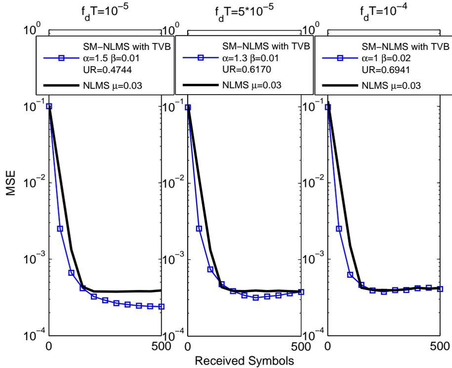
Fig. 11. MSE performance of the SM-NLMS channel estimation for Rayleigh fading channels compared with the NLMS channel estimation.  $n_p=500$ ,  $n_t=50$  and  $n_d=450$ .
