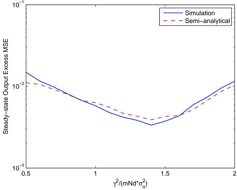
Fig. 15. Steady-state excess MSE analysis for the SM-NLMS channel estimation.
