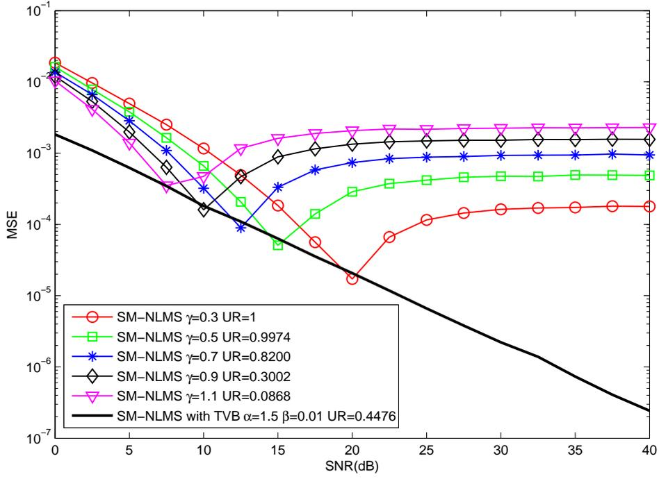
Fig. 9. SM-NLMS channel estimation MSEs versus SNR for both the fixed bound and time-varying bound for quasi-static fading channel.  $n_p=1000$ ,  $n_t=100$  and  $n_d=900$ .
