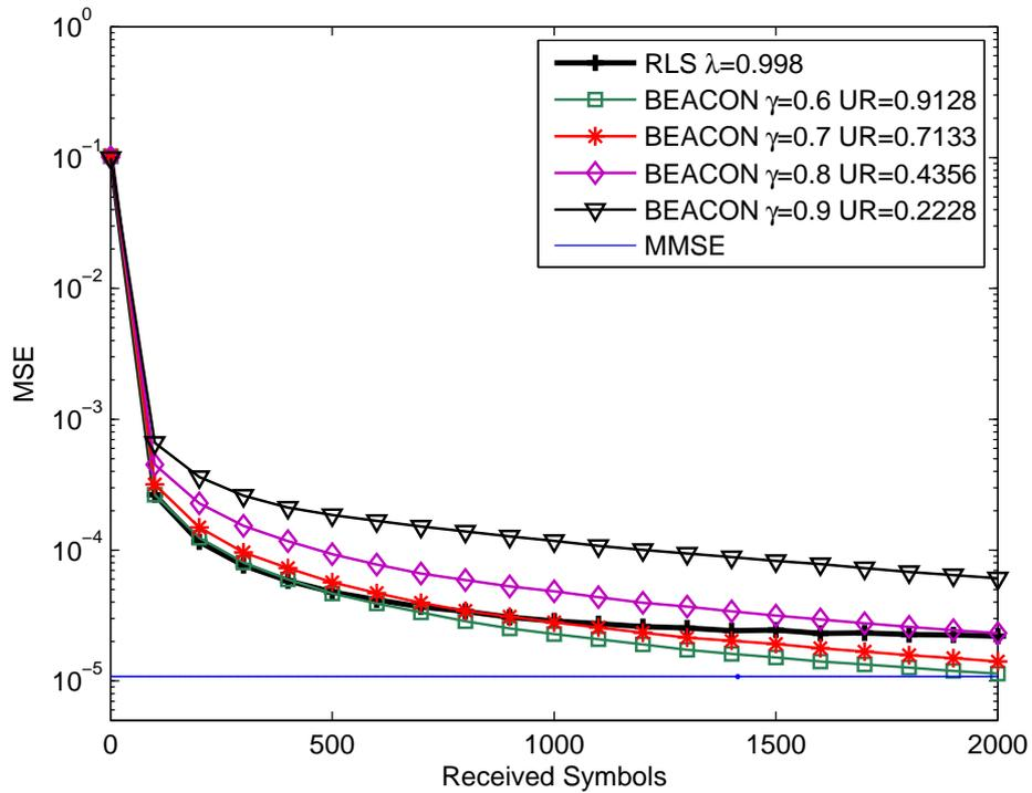
Fig. 6. MSE performance of the BEACON channel estimation of  $\mathbf{H}_d$  for quasi-static fading channel compared with the RLS channel estimation.  $n_p=2000$ ,  $n_t=100$  and  $n_d=1900$ .
