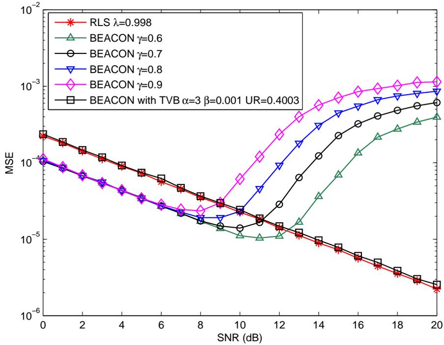
Fig. 10. BEACON channel estimation MSEs versus SNR for both the fixed bound and time-varying bound for quasi-static fading channel.  $n_p=2000$ ,  $n_t=100$  and  $n_d=1900$ .
