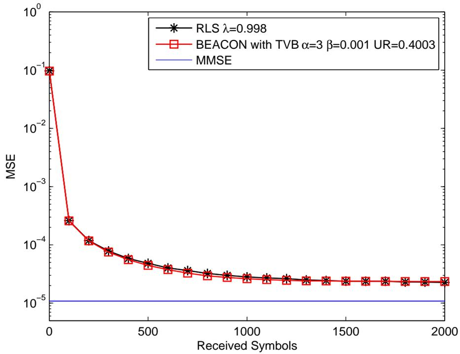
Fig. 8. MSE performance of the BEACON channel estimation with a time-varying bound for quasi-static fading channel.  $n_p=2000$ ,  $n_t=100$  and  $n_d=1900$ .
