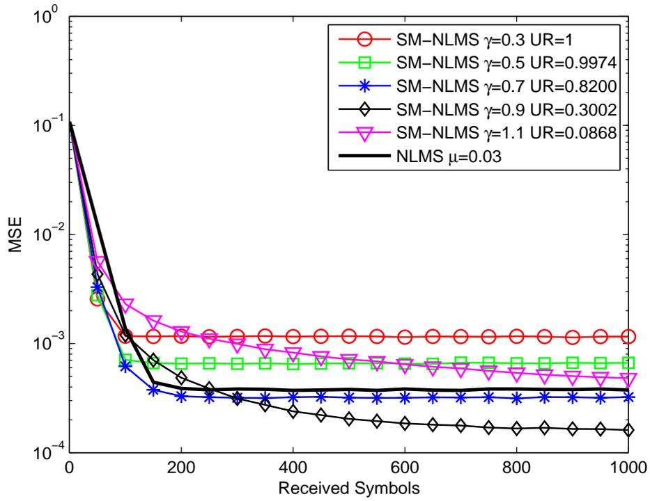
Fig. 5. MSE performance of the SM-NLMS channel estimation of  $\mathbf{H}_d$  for quasi-static fading channel compared with the NLMS channel estimation.  $n_p=1000$ ,  $n_t=100$  and  $n_d=900$ .
