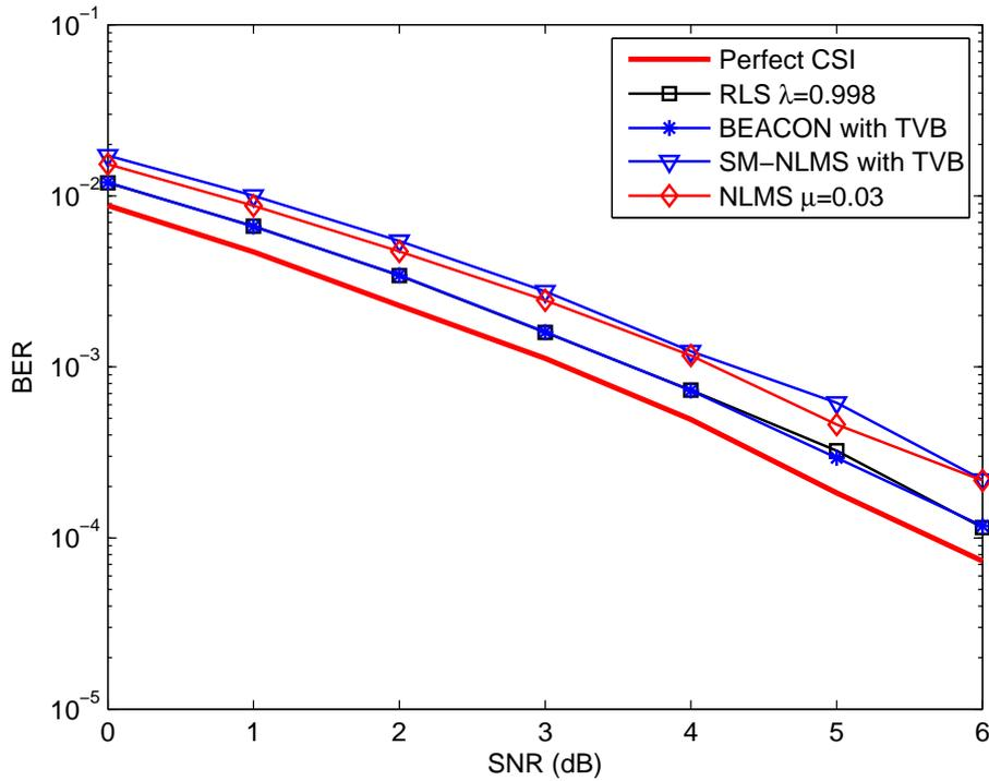
Fig. 13. BER performance of the proposed channel estimation algorithms.  $n_p=1000$ ,  $n_t=100$  and  $n_d=900$ .
