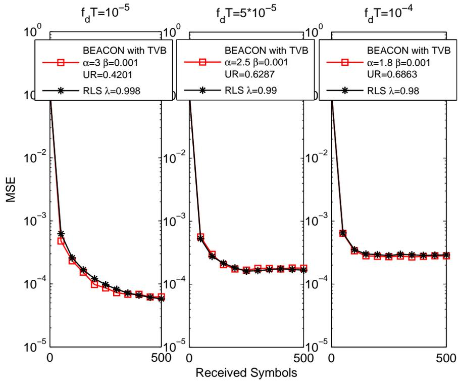
Fig. 12. MSE performance of the BEACON channel estimation for Rayleigh fading channels compared with the RLS channel estimation.  $n_p=500$ ,  $n_t=50$  and  $n_d=450$ .
