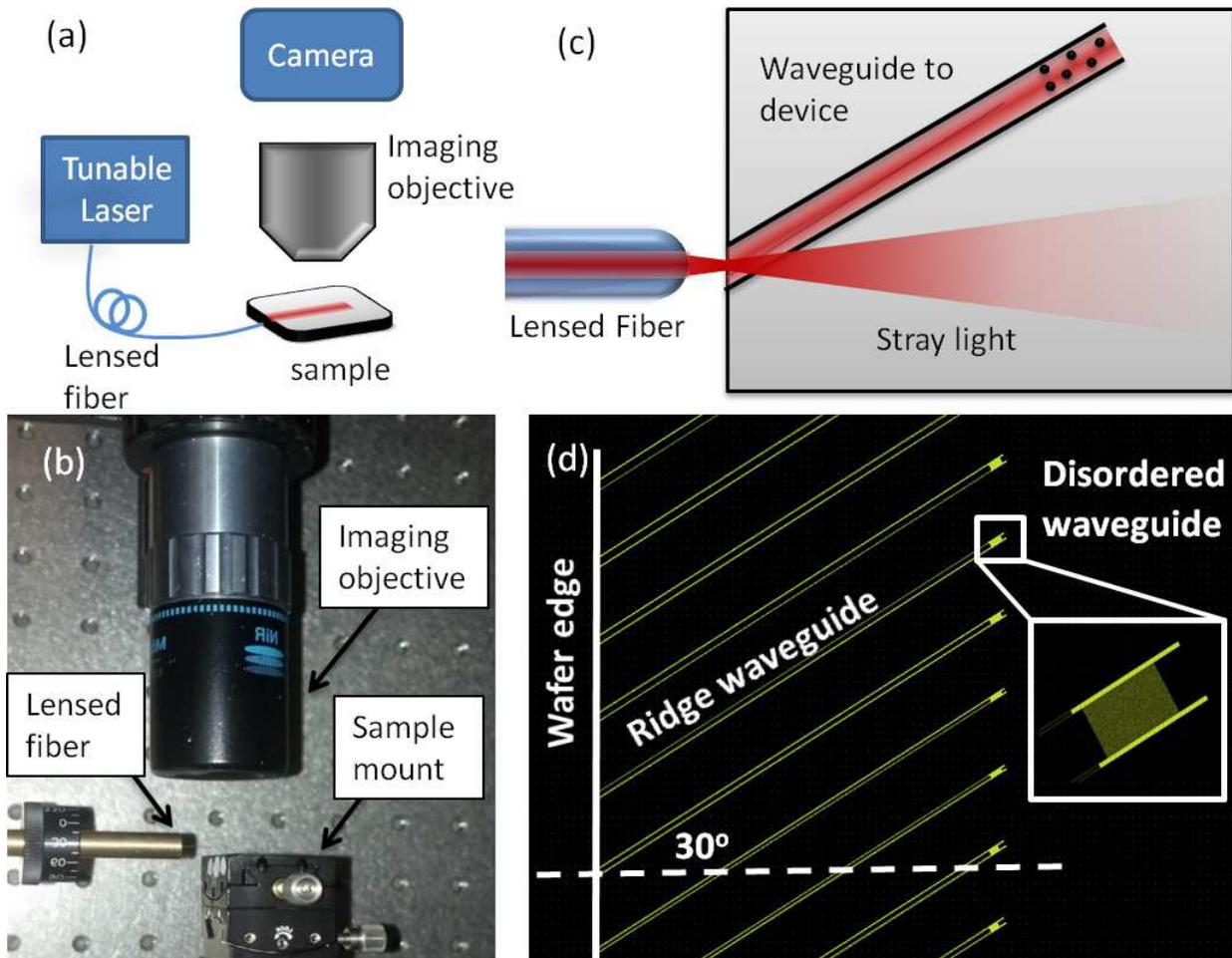
Figure S 1: **Optical measurement setup.** **a**, Schematic of experimental setup for measuring light transport inside the random waveguide. **b**, Photograph of the experimental setup. **c**, Schematic of the sample layout showing the ridge waveguides coupling the probe light from the edge of the wafer to the random waveguides with photonic crystal sidewalls. **d**, Layout of the fabricated structures studied experimentally.
