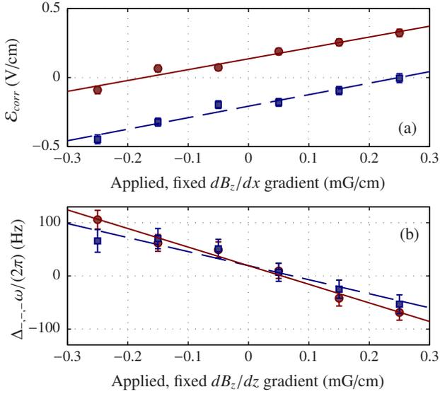
FIG. 10. (Color online) (a) Variation of  $\mathcal{E}_{corr}$  as a function of fixed  $dB_z/dx$ . (b) The variation in  $eEDM$  signal channel  $\Delta_{+,-,-}\omega$  as a function of fixed  $dB_z/dz$ . The red circles show the signal from the detector fixed in the  $+\hat{x}$  direction and the blue squares show the signal from the detector along the  $-\hat{x}$  direction.
