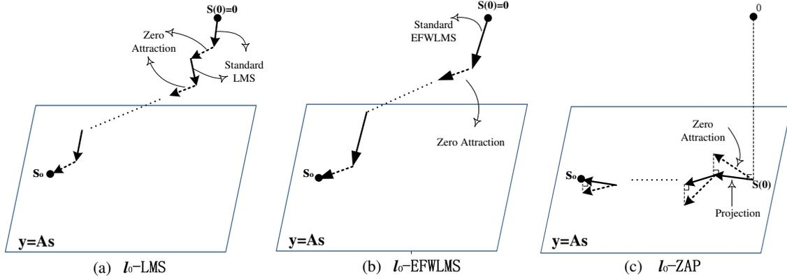
Figure 2: The updating procedures of the three methods, where  $\mathbf{s}_0$  denotes the original signal and  $\mathbf{s}(0)$  denotes the initial value. (a)  $l_0$ -LMS; (b)  $l_0$ -EFWLMS; (c)  $l_0$ -ZAP.
