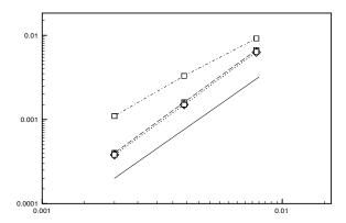
Fig. 1. Convergence in the  $L^2$ -norm plotted against the timestep  $\tau = h$ , of the stabilized (dashed line for explicit and dotted line for implicit treatment of the stabilization operator) and unstabilized (dash-dot) Crank-Nicolson method. The full line shows optimal second order convergence.
