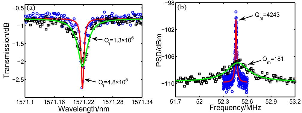
Fig. 2. Measurements for DUT1. (a) Cavity transmission spectra with different taper couplings. The transmission spectrum denoted by the blue circle with red line fitting is obtained when the taper is 400nm away from the resonator. The transmission spectrum denoted by the black square with green line fitting is obtained when the taper touches the resonator. (b) RF spectra of the breathing mode when the taper is away from (blue circle) and in contact with the resonator (black square).
