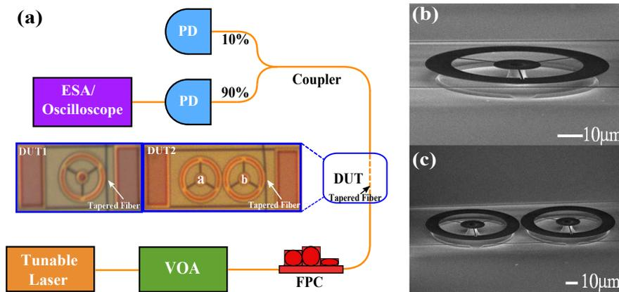
Fig. 1. (a) Experimental setup. VOA: Variable Optical Attenuator; FPC: Fiber Polarization Controller; PD: Photodetector; ESA: Electrical Spectrum Analyzer; DUT: Device Under Test. A tapered fiber is used to couple light into and out of the resonator, and it is parked on the nanostrings. The experiments are conducted under vacuum. Both single wheel resonator(DUT1) and two side-coupled wheel resonators(DUT2) are investigated. (b) SEM image of DUT1. (c) SEM image of DUT2.
