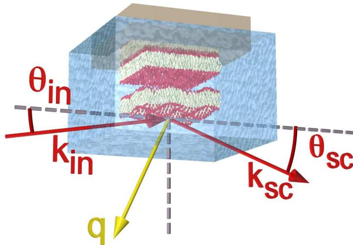
FIG. S1: Schematic view of the experimental setup for specular and off-specular reflectivity. The grazing and scattered wavevectors (resp. angles of incidence) are  $\mathbf{k}_{in}$  and  $\mathbf{k}_{sc}$  (resp.  $\theta_{in}$  and  $\theta_{sc}$ ).  $\mathbf{q}$  is the wavevector transfer.
