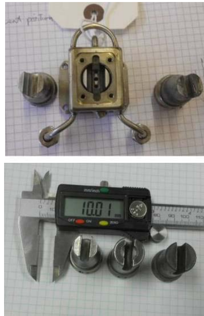
Figure 1: Modification of ISIS PD SPS: (Top) right-standard cathode with a discharge gap d=5 mm; left-modified cathode with gap d=7 mm; central-PD SPS assembling with modified cathode gap d=9 mm and the
