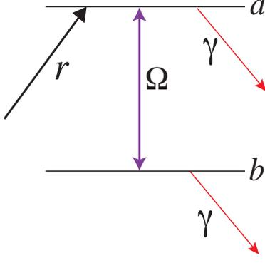
FIG. 15: Two-level model. The decay rate from the levels  $|a\rangle$  and  $|b\rangle$  is given by  $\gamma$  while the rate of populating upper level is  $r$ .
