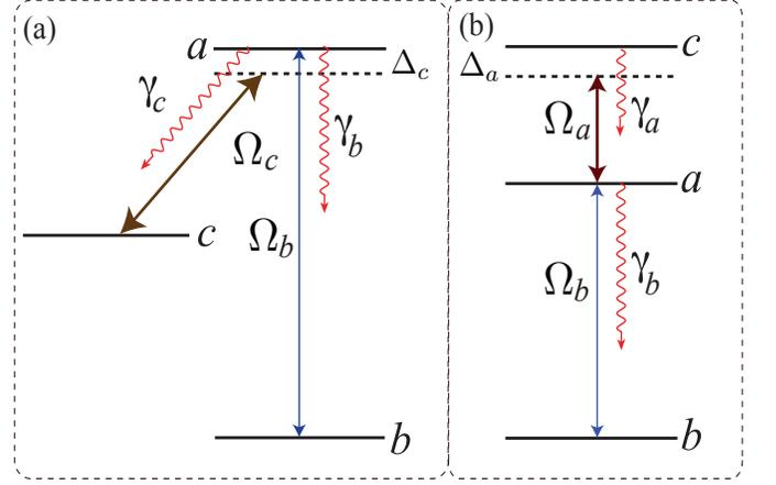
FIG. 2: Three-level atomic system in (a)  $\Lambda$  and (b)  $\Xi$  configurations.
