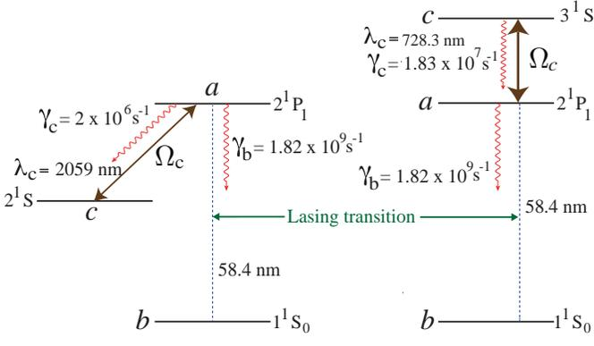
FIG. 5: Energy level diagram of He atom in  $\Lambda$  (left) and  $\Xi$  configurations (right) respectively. Lasing at 58.4nm can be enhanced using a coherent drive at 2059nm( $\Lambda$ -configuration) or 728.3nm( $\Xi$ -configuration)[51]
