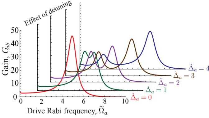
FIG. 12: Plot of steady-state gain  $G_{ab}$  as a function of the coherent drive  $\tilde{\Omega}_a$  for different choices of the detuning  $\tilde{\Delta}_a = 1, 2, 3, 4$ . Here  $\tilde{\Delta}_a$  normalized to the population transfer rate  $R_{ea}$ . Other parameters are same as Fig. 10.
