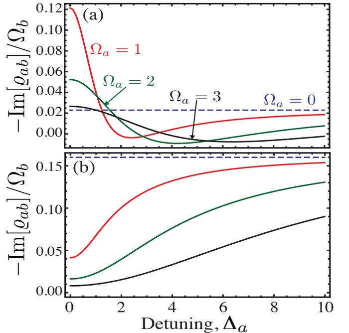
FIG. 8: Plot of  $-\text{Im}[\rho_{ab}]/\Omega_b$  as a function of the detuning  $\Delta_a$  for different values of the drive Rabi frequency  $\Omega_a$ . In (a) we have we assume incoherent pump from the lower level  $|b\rangle \rightarrow |c\rangle$  while in (b) we considered the incoherent pump from the lower level  $|b\rangle \rightarrow |a\rangle$ . The dashed line corresponds to no drive  $\Omega_a = 0$ .
