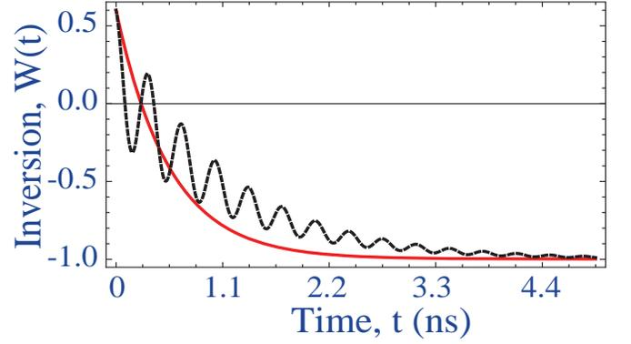
FIG. 4: Inversion  $W(t)$  in the probe transition ( $a \leftrightarrow b$ ) vs time  $t$ . Dashed black curve shows the result for  $\Omega_c = 5\gamma_b$  while solid red curve is obtained with no drive. For numerical simulation we used  $\gamma_c = 1.1 \times 10^{-3} \gamma_b$  and the initial condition  $\rho_{aa}(0) = 0.8, \rho_{bb}(0) = 0.2, \rho_{cc}(0) = \rho_{ac}(0) = \rho_{ab}(0) = 0$ .
