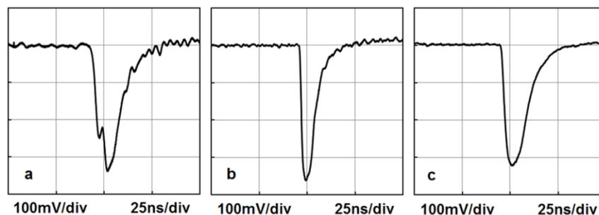
Fig. 5. Typical output signals obtained with a Fe-55 source: (a) – without a series resistor  $R_s$ ; (b) – with  $R_s = 180\Omega$ ; (c) – with  $R_s = 240\Omega$ .
