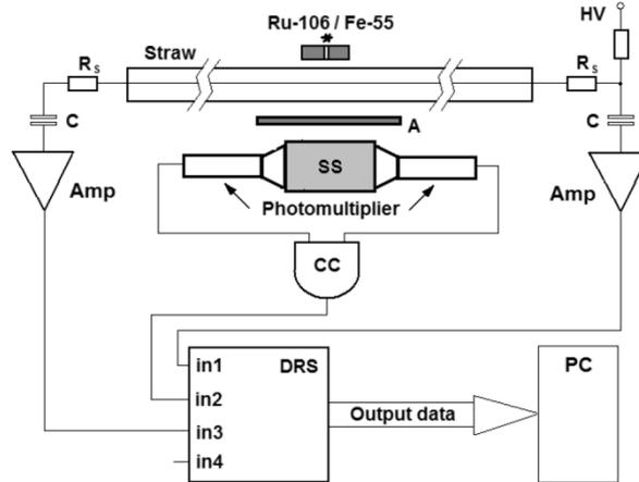
Fig. 1. A schematic view of the setup: A – absorber, SC – scintillation counter, Amp – amplifier, CC – coincidence circuit, DRS4 – Domino Ring Sampler (DRS).
