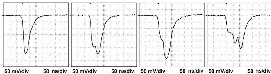
Fig. 7. Typical pulses obtained by detection of high energy electrons from a Ru-106 source. The termination is 360Ω, the anode voltage is 1.85 kV (G is  $\sim 4.5 \times 10^4$ ).
