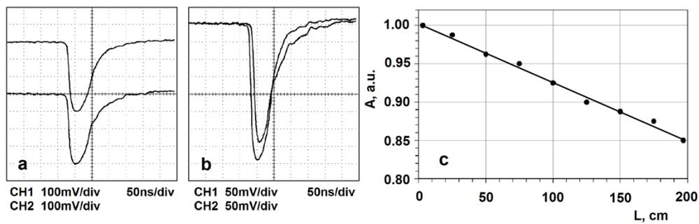
Fig. 4. (a) – Signals registered at the ends of the anode when a collimated Fe-55 source is located at the middle of the straw; (b) – Typical signals registered by an amplifier when a collimated Fe-55 source is located near the end of the straw; (c) – Signal attenuation as a function of the distance from the straw end.
