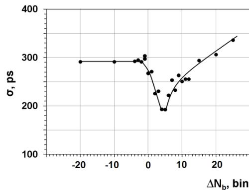
Fig.10. The longitudinal resolution as a function of the variation of the  $\Delta N_b$  near the measured value of  $N_b$ . The distance of a Ru-106 source from the straw center is 97 cm. Position of 0 (X-axis) corresponds to the primary measured value  $N_b$ .
