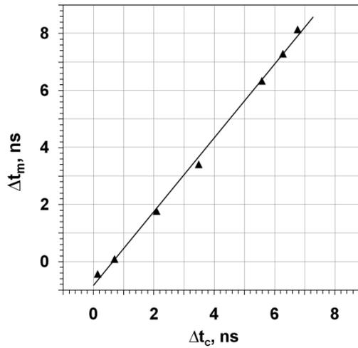
Fig. 11. The correlation between the measured ( $\Delta t_m$ ) and the calculated ( $\Delta t_c$ ) time differences along the straw.
