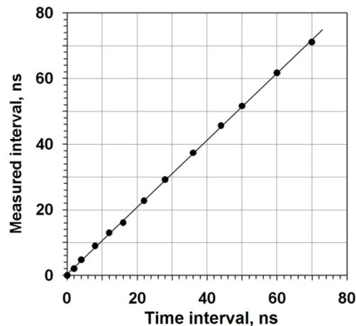
Fig. 3. The measured time interval as a function of the calibrated delay interval varied in the range of 2–70 ns (DRS4 linearity).
