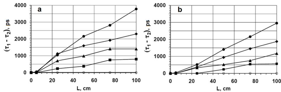
Fig. 6. A time difference between leading edges of the pair of pulses as a function of the distance of a Fe-55 source from the middle of the straw tube: (a) – termination of the straw is 120Ω; (b) – termination is 360Ω. The symbols correspond to different signal levels at the leading edge as a fraction of the peak value: 0.15 – open circles, 0.3 – filled squares, 0.45 – filled diamonds, and 0.75 – filled circles. Gas gain (G) is  $\sim 4 \times 10^4$ .
