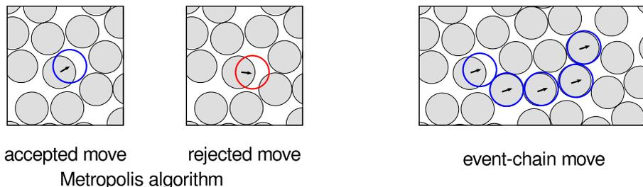
**Figure 2.** Monte Carlo moves for hard disks. *Left:* Accepted and rejected Metropolis moves. *Right:* Event-chain move. The sum of individual displacements equals a predefined value  $\ell$ . With periodic boundary conditions, the event-chain move is rejection-free.
