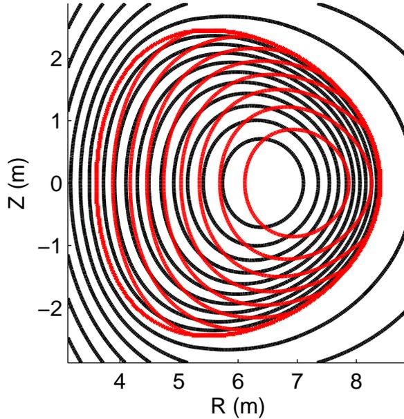
**Figure 4.** The displacement of pressure contours from magnetic surfaces in the reconstructed flowing Soloviev benchmark. Pressure shown in red.
