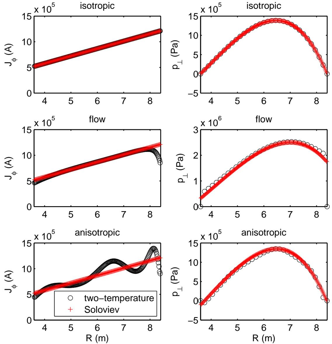
**Figure 3.** Reconstruction of analytical radial profiles using EFIT TENSOR and constraining to pressure. The difference in parallel heat transport assumptions of the analytical solution and the two temperature GCP model has resulted in a different current profile for the same pressure profile.
