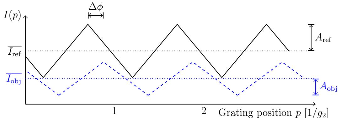
FIG. 2: Example intensity oscillations  $I(p)$  detected in a detector pixel as a function of the lateral position of grating G2. The solid line shows the reference oscillation without the object while the dashed line shows the resulting oscillation with object.  $\bar{I}$  are the mean values while  $A$  are the amplitudes of the oscillations.  $\Delta\phi$  is the phase difference between the oscillations and is the measurement parameter for the differential-phase image.
