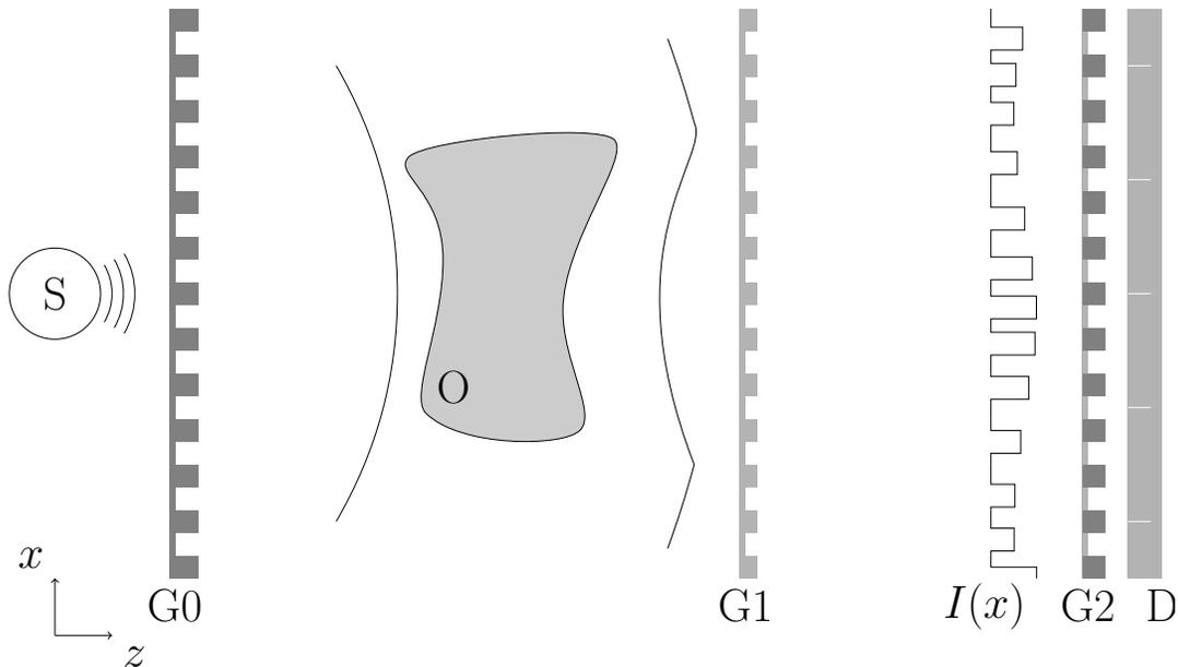
FIG. 1: Sketch of the used Talbot-Lau Interferometer with X-ray source S, source grating G0, a sample O, the phase grating G1, the analyser grating G2, and a pixelated detector D.  $I(x)$  illustrates the idealized, monoenergetic Talbot intensity pattern, produced by G1 and distorted by the object.
