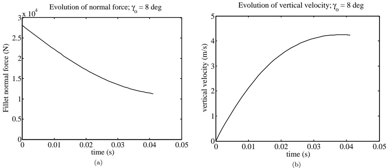
FIG. 4: Simulation results for entry angle  $\gamma_o = 8^\circ$ . Contact duration is only 0.041 s but contact persists until the top of the fillet is reached. a) Normal force decreases from 28 kN to 11 kN, and the average force of 14 kN during the last half of contact acts nearly horizontally. b) A substantial portion (> 80%) of the vertical velocity at launch is achieved in less than half the contact time because the normal force acts mostly in the vertical direction during this period.
