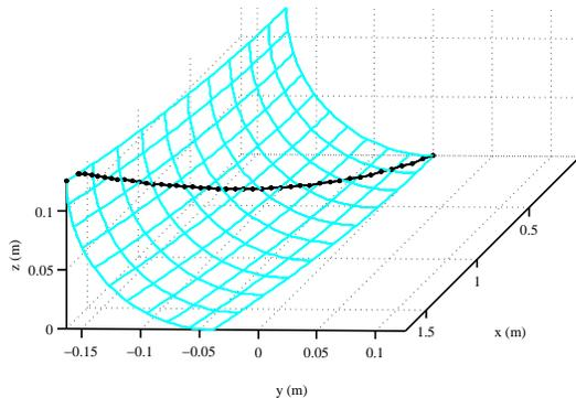
FIG. 5: Simulation results ( $x$  axis not to scale) for entry angle  $\gamma_o = 8^\circ$ . Luge 3D path rises to top of fillet as inner wall turns away from initial direction. Loss of contact occurs when the positive normal curvature vanishes at top of fillet where it meets the cylindrical inner wall.
