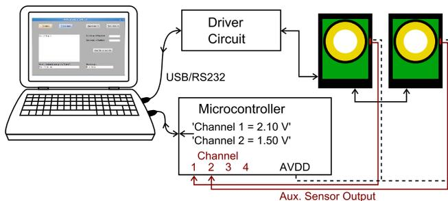
FIG. 2. (Color online) Outline of the communication scheme. The motor driver circuit and the microcontroller communicate with the control program via virtual USB serial ports. The motor system and microcontroller share the same 5 V power supply. The auxiliary sensors output a voltage directly to the microcontroller.
