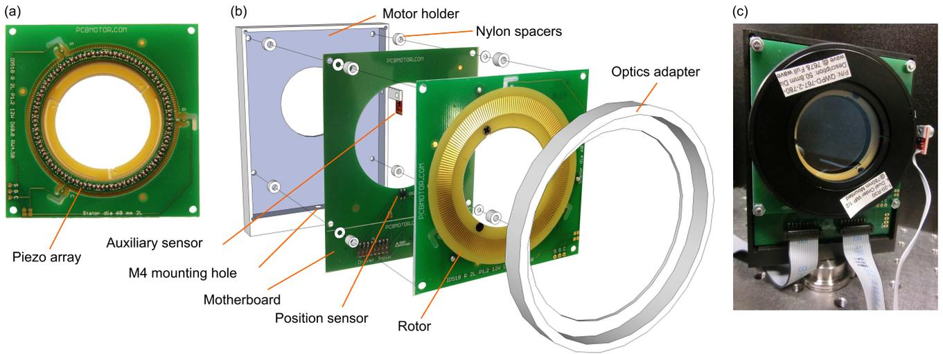
FIG. 1. (Color online) (a) The PCB stator. (b) The exploded rotator motor with rotor mounted. Ref. 9 provides mechanical drawings for the motor holder and the optics adapter. (c) The assembled rotator; video showing rotator operation (enhanced online)[URL: [www.physics.otago.ac.nz/staff\\_files/nk/files/movie1.mp4](http://www.physics.otago.ac.nz/staff_files/nk/files/movie1.mp4)]. .
