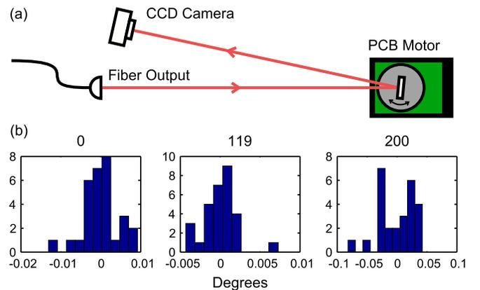
FIG. 3. (Color online) (a) Setup for measuring position repeatability for the motor. A collimated laser beam is reflected onto a CCD camera by a mirror mounted perpendicular to the motor. Beam position is determined using a Gaussian fit. (b) Histograms of repeatability data for three different points (0, 119, 200) on the code wheel.  $0^\circ$  indicates the mean position for each data set.
