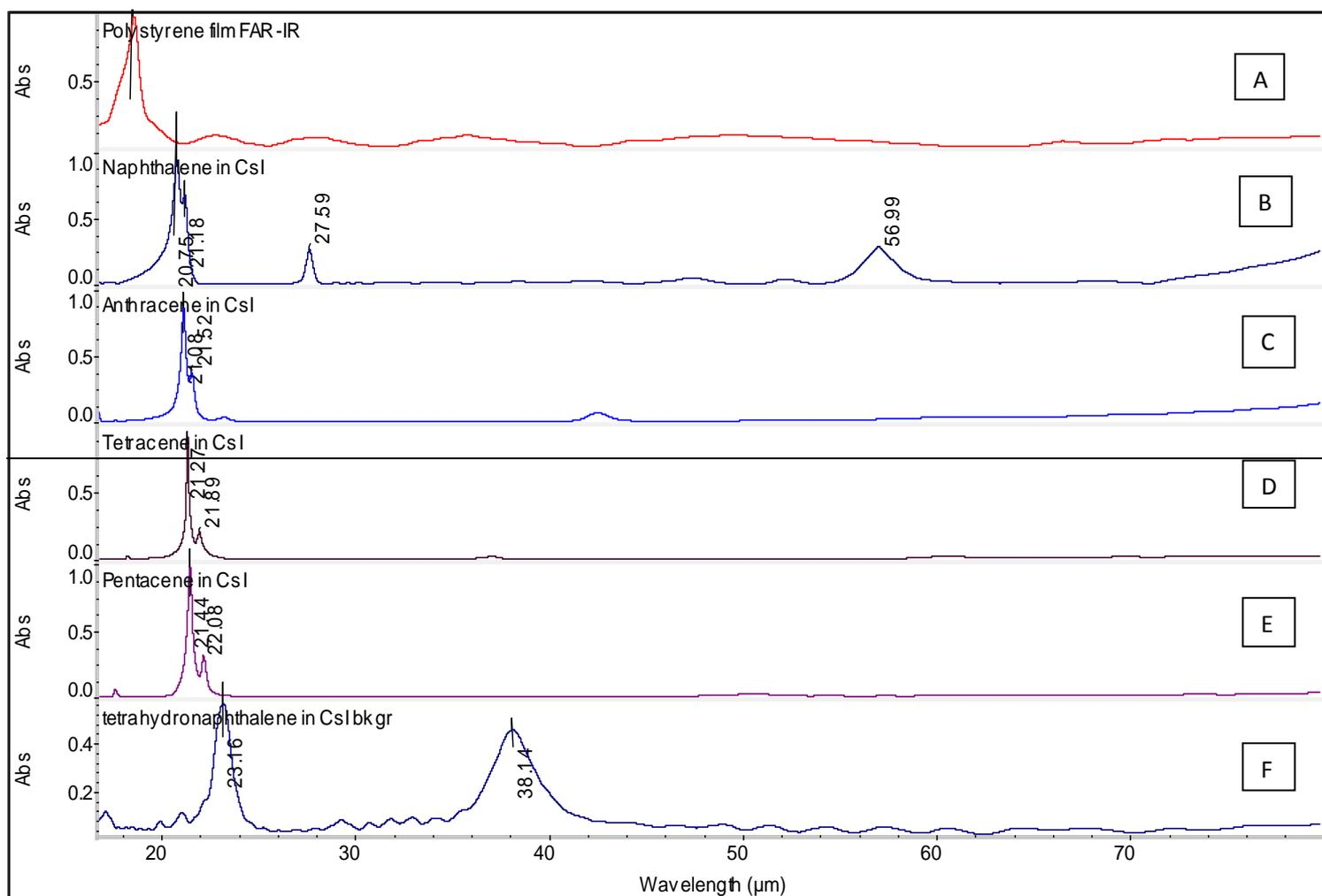
Figure 6 – FT-IR spectra in the FAR-INFRARED between 16.0 and 80.0  $\mu\text{m}$  of a series of acenes with the exclusion of the first spectrum on top which is due to polystyrene (A). The latter is followed from top to bottom by the spectrum of B= naphthalene, C= anthracene, D= tetracene, E= pentacene and F= tetrahydronaphthalene.
