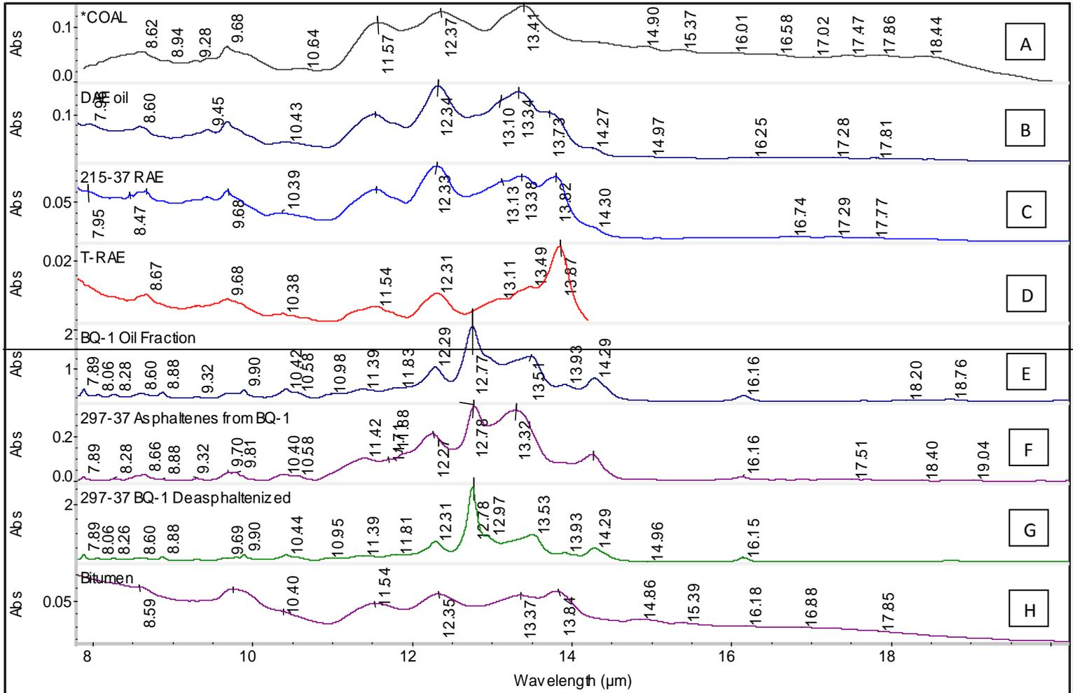
Figure 4 – FT-IR spectra between 8.0 and 20.0  $\mu\text{m}$ . From top to bottom are shown respectively the spectra of **A** = Coal; **B** = DAE; **C** = RAE; **D** = T-RAE; **E** = BQ-1; **F** = Asphaltenes from BQ-1; **G** = Deasphaltenized BQ-1; **H** = Bitumen.
