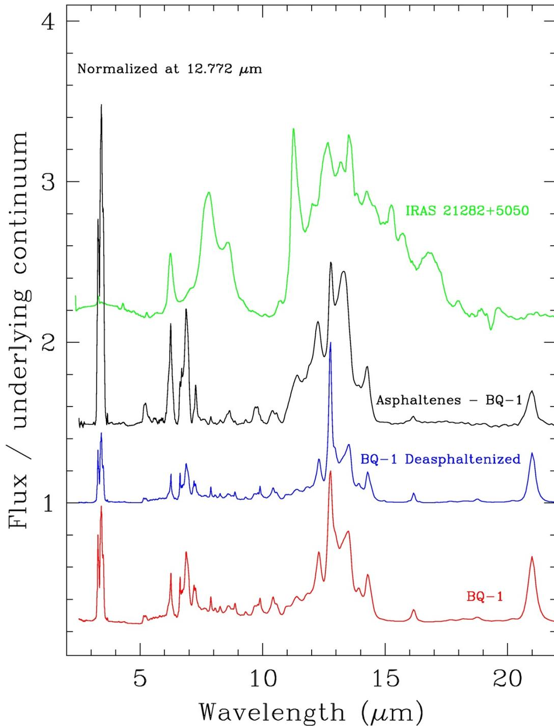
Figure 13. Laboratory spectra for BQ-1 (in red), Deasphaltenized-BQ-1 (in blue), and Asphaltenes (in black) in the range  $\sim 3$ - $22 \mu\text{m}$  in comparison with the Infrared Space Observatory spectra (Flux divided by the underlying continuum, see text) of the young PN IRAS 21282+5050 (in green). Note that the PN spectrum has been smoothed (with a 75-point box car filter) in order to be compared with to the laboratory spectra.
