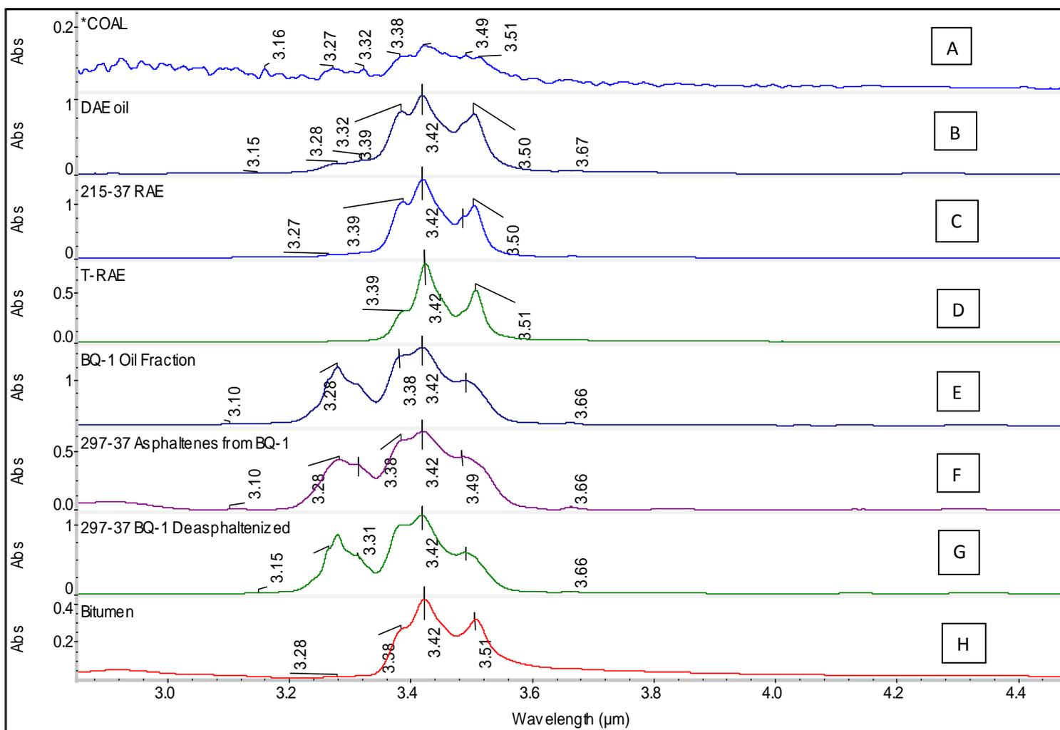
Figure. 1 – FT-IR spectra in the C-H stretching band region. From top to bottom are shown respectively the spectra of **A** = Coal; **B** = DAE; **C** = RAE; **D** = T-RAE; **E** = BQ-1; **F** = Asphaltenes from BQ-1; **G** = Deasphaltenized BQ-1; **H** = Bitumen.
