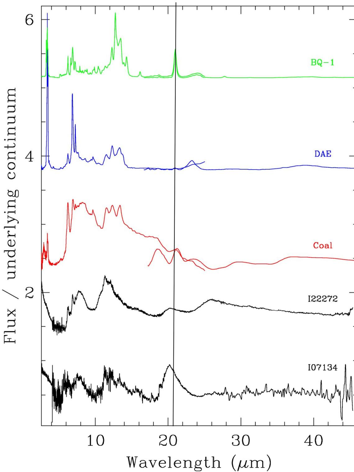
Figure 12. Laboratory spectra for BQ-1 (in green), DAE (in blue), and coal (in red) in the range 2-50  $\mu\text{m}$  in comparison with the Infrared Space Observatory spectra (Flux divided by the underlying continuum, see text) of the PPNe IRAS 22272+5435 and IRAS 07134+1005 (both in black). Note that this time the PPNe spectra have not been smoothed. Note that the far-infrared spectra were scaled to the mid-infrared ones (e.g., by using the 21  $\mu\text{m}$  feature that overlaps).
