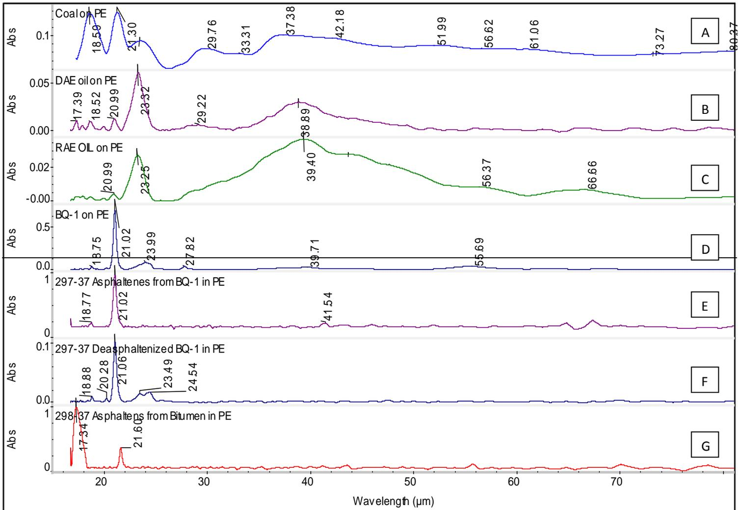
Figure 5 – FT-IR spectra in the FAR-INFRARED between 16.0 and 80.0  $\mu\text{m}$ . From top to bottom are shown respectively the spectra of **A** = Coal; **B** = DAE; **C** = RAE; **D** = BQ-1; **E** = Asphaltenes from BQ-1; **F** = Deasphaltenized BQ-1; **G** = Asphaltenes from bitumen.
