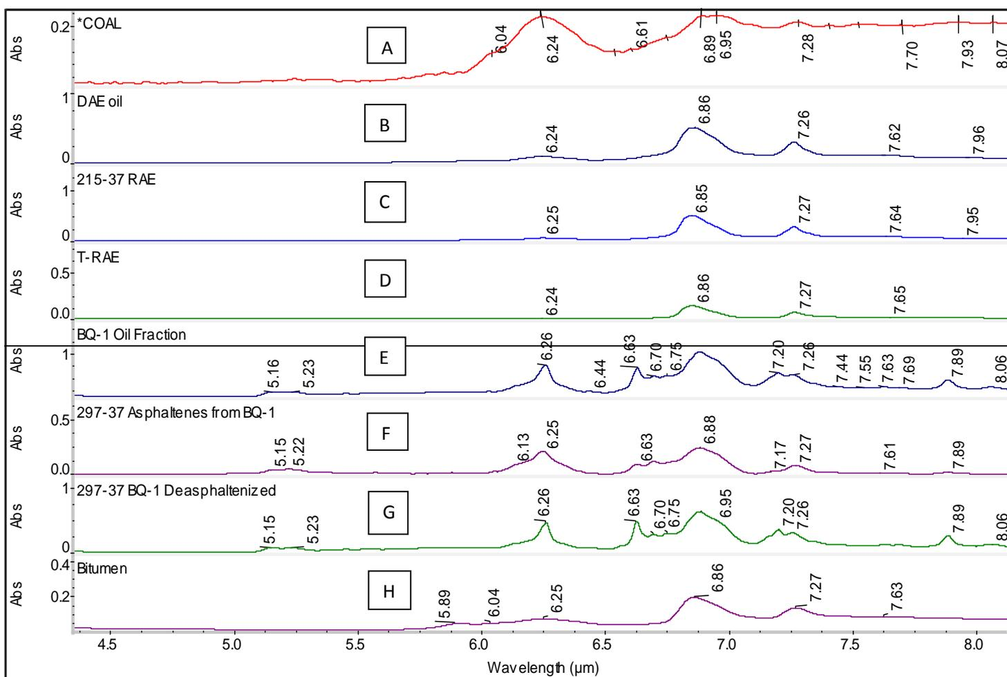
Figure 3 – FT-IR spectra between 4.5 and 8.0  $\mu\text{m}$ . From top to bottom are shown respectively the spectra of **A = Coal**; **B = DAE**; **C = RAE**; **D = T-RAE**; **E = BQ-1**; **F = Asphaltenes from BQ-1**; **G = Deasphaltenized BQ-1**; **H = Bitumen**.
