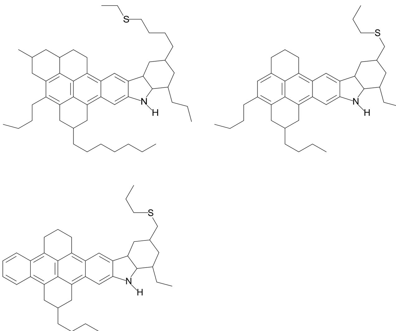
*Figure 9 – Petroleum asphaltene molecular models with an anthracene or tetracene “core” from BQ-1. The basic asphaltene structures were taken from Mullins et al. (2007) and modified slightly to take into account the current experimental data suggested by the far infrared spectra. These chemical structures represent the “average” possible structures of asphaltenes extracted from the petroleum fraction BQ-1.*
