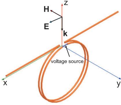
Fig. 4. Active omega particle showing zero forward scattering at 1.8 GHz.
