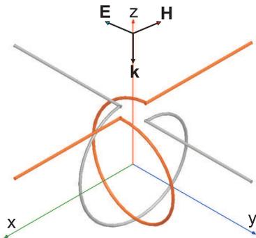
Fig. 2. Uniaxial chiral particle showing zero backscattering at 1.8 GHz. The two elements are drawn with different colors only for clarity.
