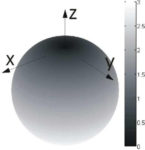
Fig. 1. Scattering directivity pattern (absolute values) for an incident plane wave propagating along the  $-z$ -direction exciting a moving particle with the polarizabilities satisfying  $\alpha_{ee} = \frac{1}{\eta_0} \alpha_{mm}$  (or an omega particle with  $-\alpha_{ee} - \frac{2}{\eta_0} \alpha + \frac{1}{\eta_0} \alpha_{mm} = 0$ ).
