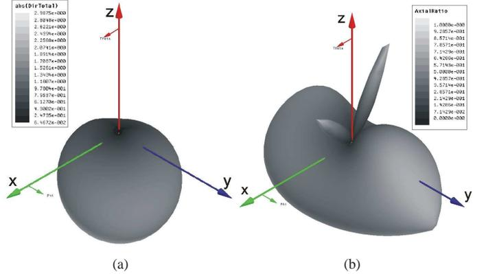
Fig. 3. Scattering directivity pattern (a) and axial ratio pattern (b) for the chiral particle of Fig. 2 at 1.8 GHz (absolute values).
