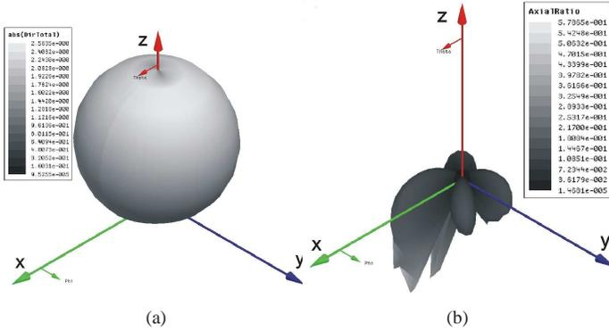
Fig. 5. Scattering directivity pattern (a) and axial ratio pattern (b) for the active omega particle of Fig. 4 at 1.8 GHz (absolute values).
