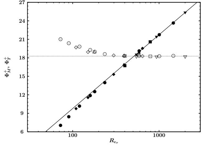
FIG. 1: Evolution with the friction Reynolds number  $R_{e\tau}$  of the mean shear  $\Phi_M^+$  (open symbols) and turbulent  $\Phi_T^+$  (filled symbols) contributions to the nondimensionalized dissipation function. —, [Eq. (0.1)]. Symbols in Table I.
