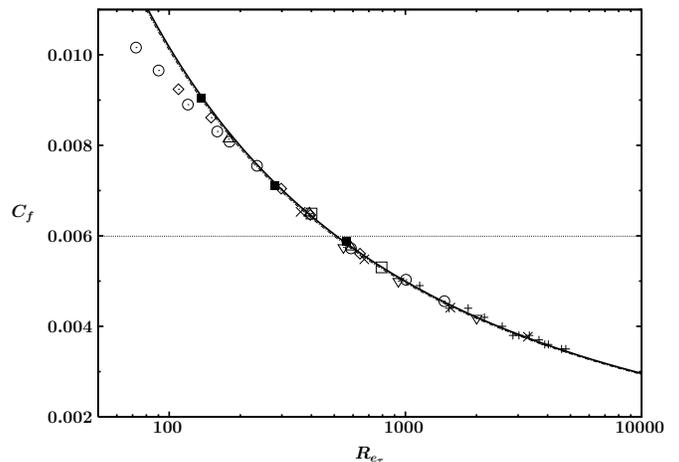
FIG. 4: Skin-friction coefficient. —, logarithmic friction law from Eq. (0.2); - - - - - best fit of boundary layer measurements of Österlund *et al.* (Ref. 19). Other symbols are the same as in Fig. 3.
