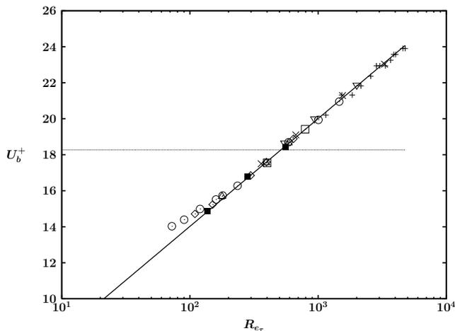
FIG. 3: Reynolds number evolution of  $U_b^+$ , the bulk velocity normalized by friction velocity. Experimental data: (+), Zanon *et al.* (Ref. 14); ( $\times$ ), Bakken *et al.* (Ref. 15); ( $\blacksquare$ ) DNS results of Spalart (Ref. 20); —, [Eq. (0.2)]. Other symbols are in Table I.
