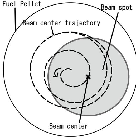
Fig. 3 Spiraling HIB. The Spiraling beam axis motion provides a sufficiently low HIBs illumination nonuniformity during the HIBs pulse duration.
