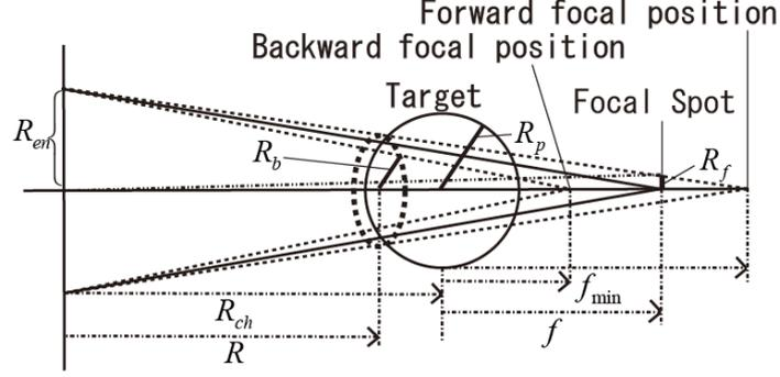
Fig. 4 A HIB illuminating on a fuel target.  $\text{Pb}^+$  ion HIBs are employed with the mean particle energy of 8 GeV. The beam radius at the entrance of a reactor chamber wall  $R_{en}$  is 35 mm, and the reactor chamber radius  $R_{ch}$  is 5 m;  $R_b$  is the beam radius on a target.
