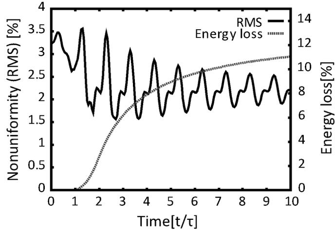
Fig. 10 Histories of the spiraling HIBs illumination nonuniformity (the solid line) and the illumination loss (the dotted line). The spiraling HIB radius changes at  $t=1.3t$  from the initial beam radius of 3.1mm to 3.0mm.
