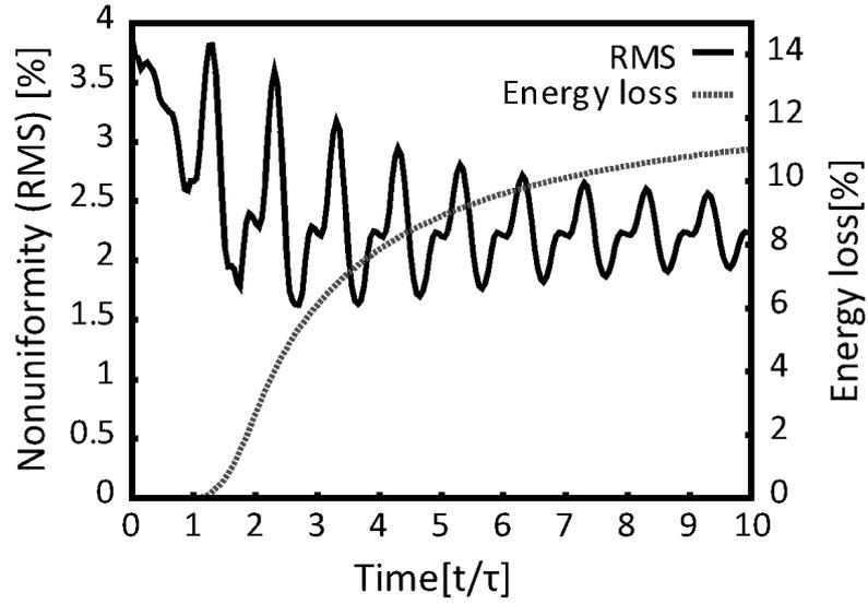
Fig. 6 Histories of the spiraling HIBs illumination nonuniformity (the solid line) and the illumination loss (the dotted line). The spiraling HIBs provide a sufficiently uniform deposition uniformity in HIF.
