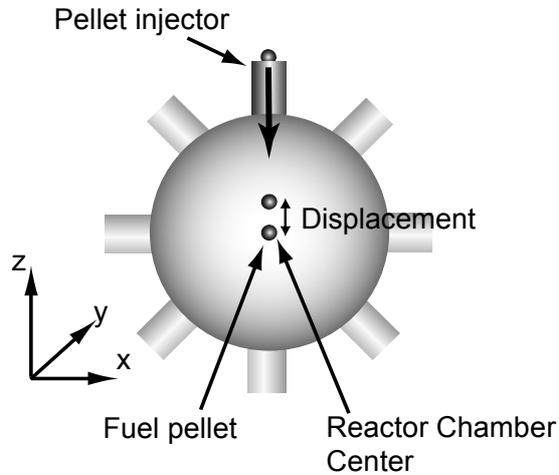
Fig. 11 Target alignment error in a fusion reactor.
