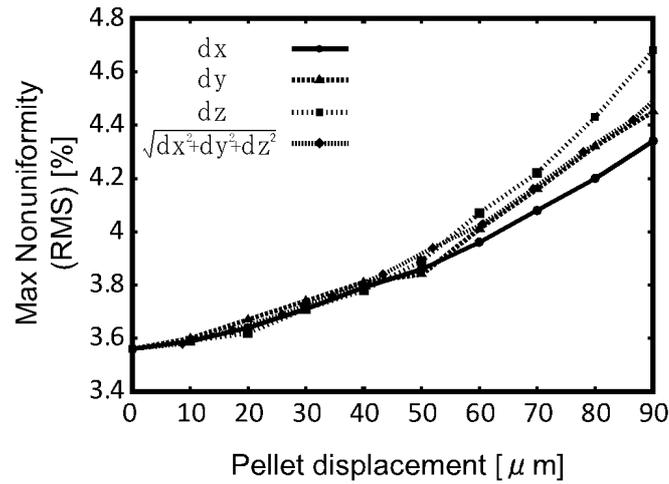
Fig. 12 The relation between the pellet displacement and the maximal *rms* nonuniformity in the best case, in which each HIB radius changes from 3.1 mm to 3.0 mm at  $t = 1.3\tau$ . The maximal *rms* nonuniformity is less than 4.5 % for the pellet displacement less than about 80  $\mu\text{m}$ .
