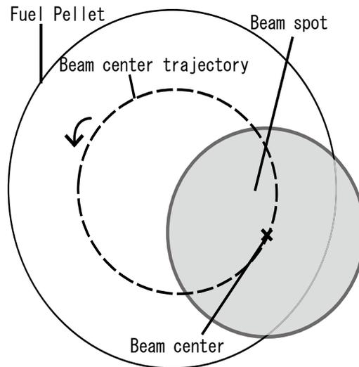
Fig. 2 A wobbling beam illumination on a direct-driven spherical target.
