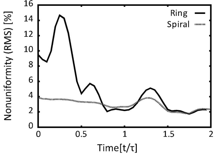
Fig. 5 Histories of energy deposition nonuniformities for the circularly moving axes (solid line) and for the spiraling HIBs. The spiraling HIB-axis motion realizes a rather low HIBs illumination nonuniformity.
