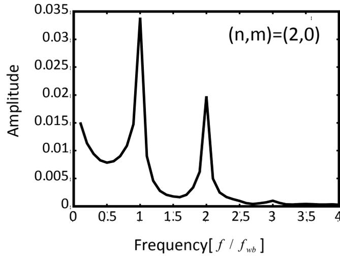
Fig. 9 Spectrum of the mode (2, 0) in its frequency space. The frequency  $f_{wb}$  is the wobbling HIB frequency. The small nonuniformity of the HIBs energy deposition has the same frequency  $f_{wb}$  of the wobblers and also the double frequency  $2f_{wb}$ .
