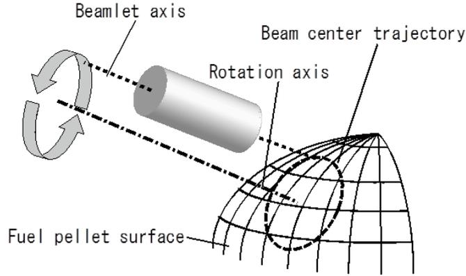
Fig. 1 The schematic diagram of wobbling HIB illumination.
