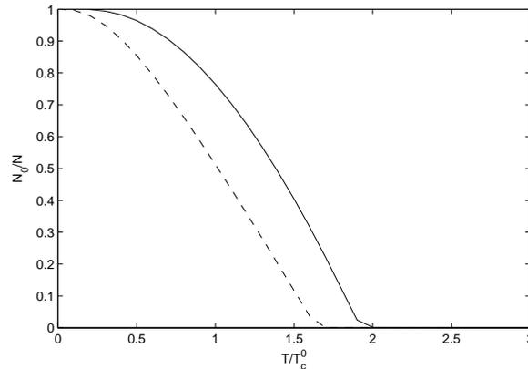
**Figure 8.** Condensate fraction  $N_0/N$  vs  $T/T_c^0$  for fixed  $\Lambda = 32$ . The solid and dashed lines show condensate fraction for  $N = 10^4$  and  $N = 10^5$ , respectively. Logarithmic scale is used for  $\Lambda$  axis. The other parameters are the same as Fig. 2.
