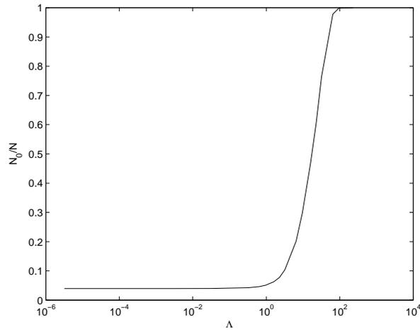
**Figure 9.** Condensate fraction  $N_0/N$  vs the strength of the Dirac  $\delta$  potential  $\Lambda$  for  $N = 10^4$  at  $T = T_c^0$ . The logarithmic scale is used for  $\Lambda$  axis. The other parameters are the same as Fig. 2.
