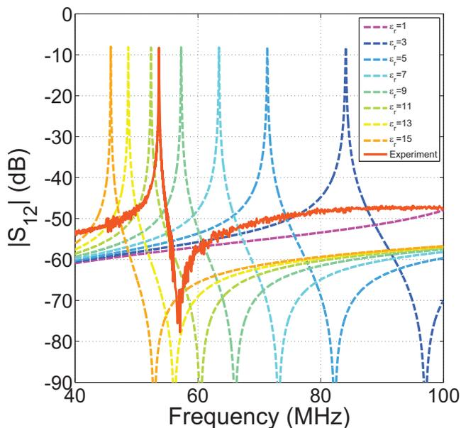
FIG. 4. The effect of substrate dielectric constant on the resonance frequency of the fundamental mode. The solid line shows the experimental resonance of the YBCO spiral on sapphire substrate and the dashed lines are the results of HFSS simulation of a perfect metal spiral of the same geometry with varying dielectric constant in the substrate.
