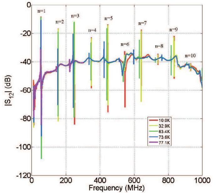
FIG. 3. Transmission spectrum of the spiral resonator below 1GHz at different temperatures. Ten modes, each with potential to create negative effective permeability, are shown.”
