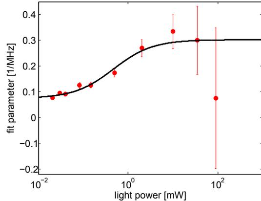
FIG. 4: Points: Fit parameter  $a/\gamma_2^{\text{intr}}$  for different light powers. The uncertainties on the points equals the 68% confidence intervals for the fit parameters  $a(P)/\gamma_2^{\text{intr}}$  calculated from the non-linear least squared fit of the measured widths to Eq. (9). Line: Weighted fit of  $a(P)/\gamma_2^{\text{intr}}$  to the function  $a_1 P / (1 + P/b_1) + c_1$ .
