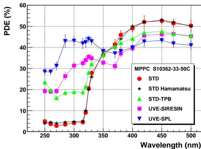
**Figure 3.** PDE as a function of wavelength for the four SiPM prototypes considered in this study. The typical PDE values of the standard MPPC S10362-33-50C from Hamamatsu are shown for comparison. These measurements were performed at  $25^\circ\text{C}$  and include effects of cross-talk and after-pulses.
