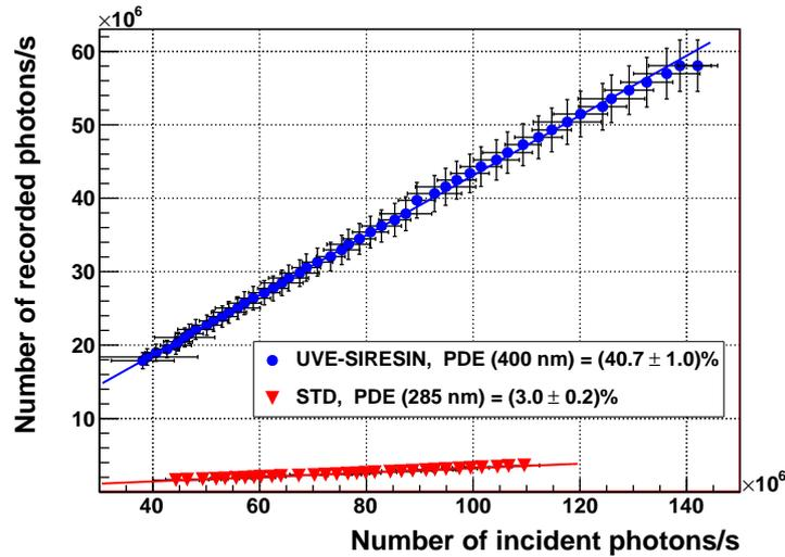
**Figure 2.** Number of recorded photons in the UVE-SIRESIN and STD SiPM prototypes as a function of the number of incident photons, measured respectively at  $400 \text{ nm} \pm 5 \text{ nm}$  and at  $285 \text{ nm} \pm 5 \text{ nm}$ . The PDE is determined from the linear fit to the data.
