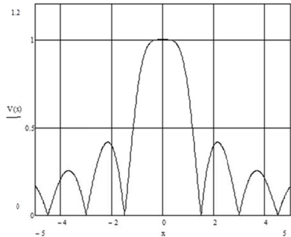
Fig.3. Distribution of spatial coherence for one-mode He-Ne laser for  $r=300$ mm,  $l=0,1$ mm.
