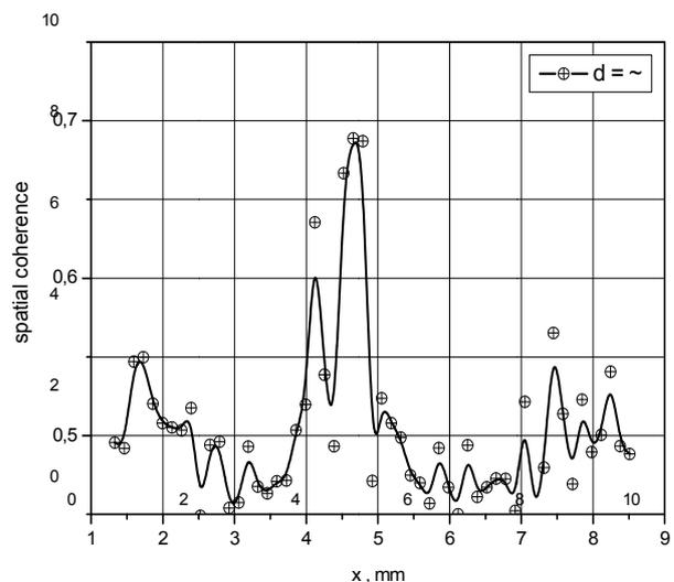
Fig.4. Spatial coherence distribution for the many-mode He-Ne laser without spatial filtration
