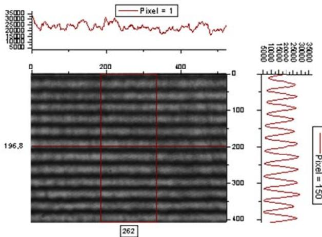
Fig.1. Luminosity distribution in a 16-bit code for longitudinal (top) and transversal (on the right) cross sections in width 1 and 150 pixel correspondently. Along x-y axes there are phase planes in pixels, along z-axis - luminosity of interference patterns in bits.
