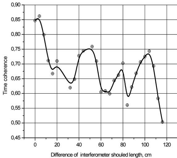
Fig.6. Time coherence measurement for two-mode He-Ne laser
