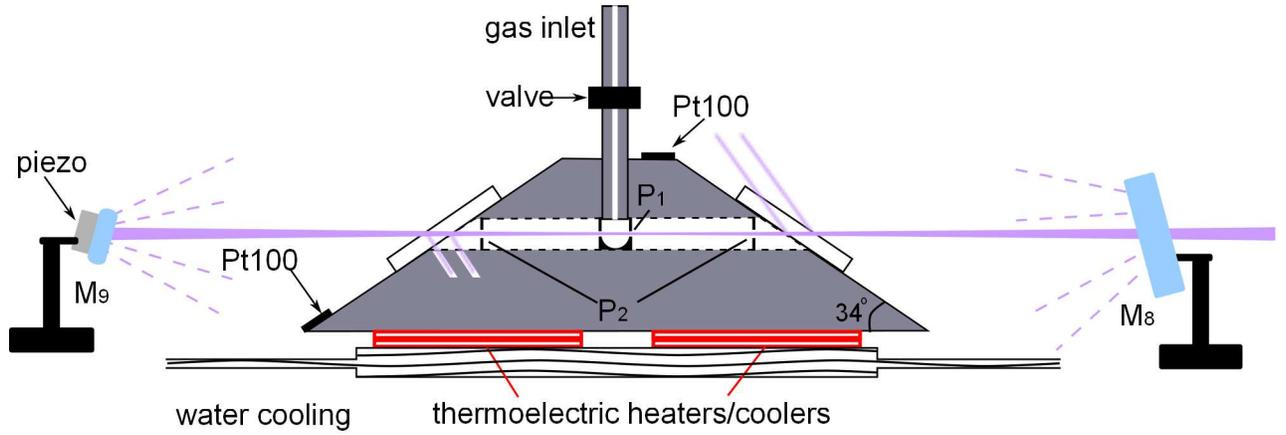
FIG. 2. Side view of the RB-scattering cell. The UV beam enters the enhancement cavity through mirror  $M_8$ .  $P_1$  and  $P_2$  are pinholes for blocking photons scattered from the mirrors and the windows. Pt100 elements are temperature sensors.
