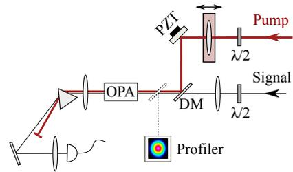
Fig. 1: (Color online) Experimental configuration of the OPA. PZT: piezoelectric transducer, DM: dichroic mirror,  $\lambda/2$ : half-wave plates.
