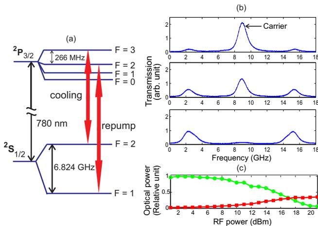
FIG. 1. (a) Partial atomic level structure of  $^{87}\text{Rb}$  with cooling and repump transitions indicated. (b) Fabry-Perot interferometer optical transmission spectra of the fiber EOM output at a driving frequency of 6.42 GHz and driving powers of 9 dBm (top), 15 dBm (center), and 21 dBm (bottom). (c) Optical power of carrier (circles) and a first-order sideband (squares) as function of rf driving power of the EOM.
