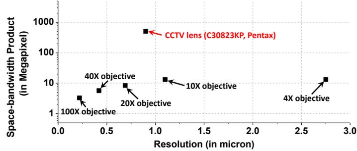
Fig. 7 The SBP-resolution summary for microscope objectives and the proposed system.
