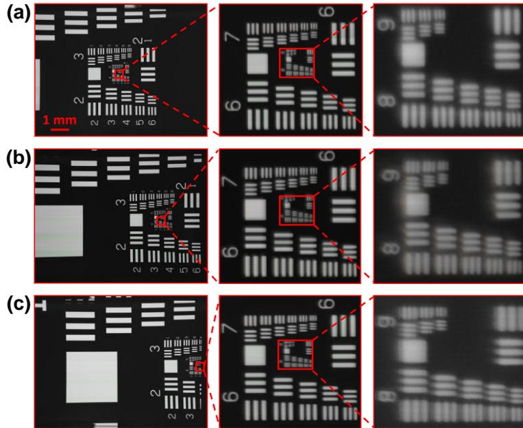
Fig. 3. USAF resolution target acquired by the proposed 0.54 gigapixel microscopy system. The effective FOV is about  $10\ \text{mm} * 7.5\ \text{mm}$ , with  $26400\ \text{pixels} * 20400\ \text{pixels}$  across the entire image. The imaging performance at the (a) center, (b) 50% away from center and (c) 95% away from center. The line widths of group 9, element 1, 2 and 3 are  $0.98\ \mu\text{m}$ ,  $0.87\ \mu\text{m}$  and  $0.77\ \mu\text{m}$  respectively.
