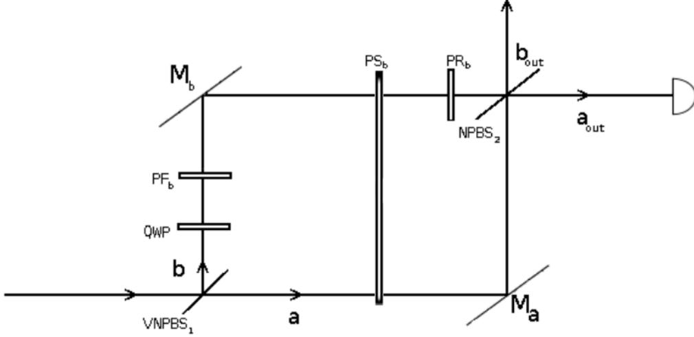
Figure 1: Schematic diagram of the experiment: A vertically polarized beam of classical light passes through a Mach-Zehnder interferometer.  $PF_b$  in path  $b$  is a polarization flipper that converts  $V$  to  $H$ .  $PS_b$  is a phase shifter and  $PR_b$  is a polarization rotator in path  $b$ .
