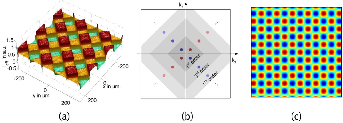
**Figure 1.** Schematics describing a multiperiodic 2D staircase lattice; (a): surface plot of the effective intensity calculated by series expansion up to an order of ten, (b): presentation of the relevant spatial frequencies, (c) periodic square lattice as the basis structure of each expansion term.
