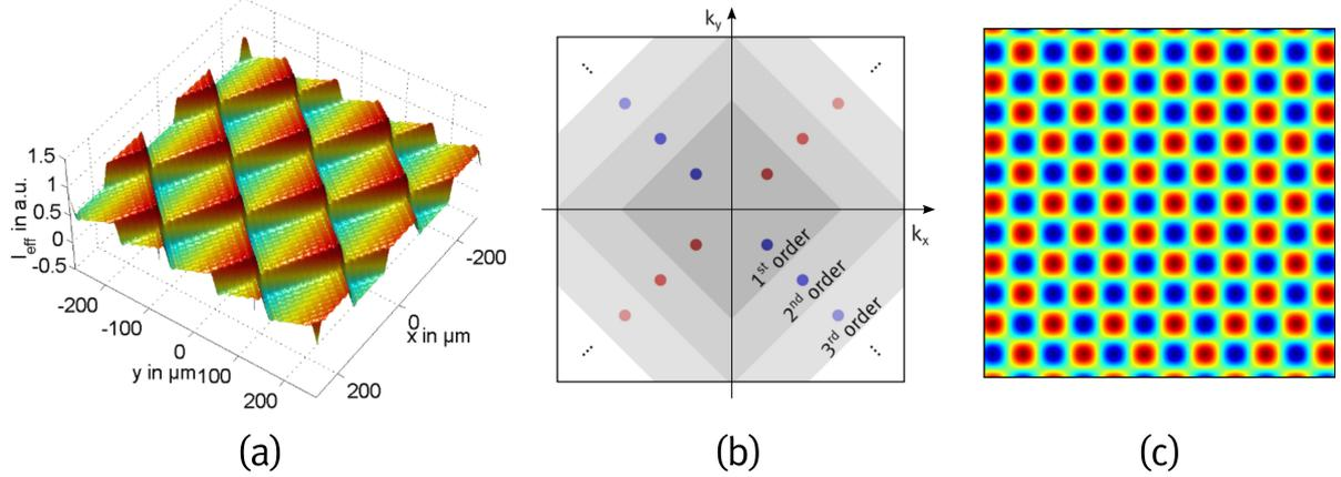
**Figure 3.** Schematics describing a multiperiodic 2D ratchet lattice; (a): surface plot of the effective intensity calculated by series expansion up to an order of ten, (b): presentation of the relevant spatial frequencies, (c) periodic square lattice as the basis structure of each expansion term.
