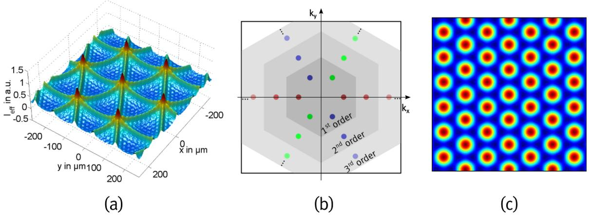
**Figure 2.** Schematics describing a multiperiodic 2D wire mesh lattice; (a): surface plot of the effective intensity calculated by series expansion up to an order of ten, (b): presentation of the relevant spatial frequencies, (c) periodic hexagonal lattice as the basis structure of each expansion term.
