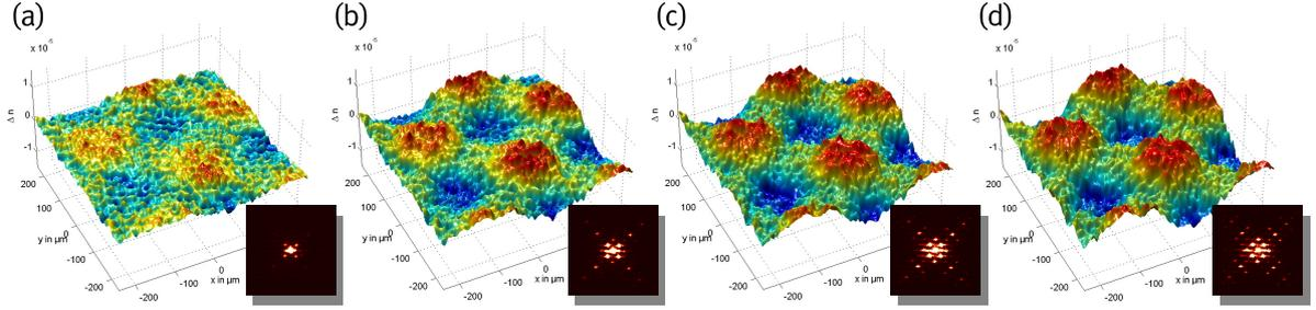
**Figure 6.** Time development of the rectangularly modulated refractive index structure. The detailed illumination times are (a)  $t_1 = 20$  s, (b)  $t_2 = 80$  s, (c)  $t_3 = 140$  s, (d)  $t_4 = 200$  s. Respective insets present corresponding intensity distributions in far field.
